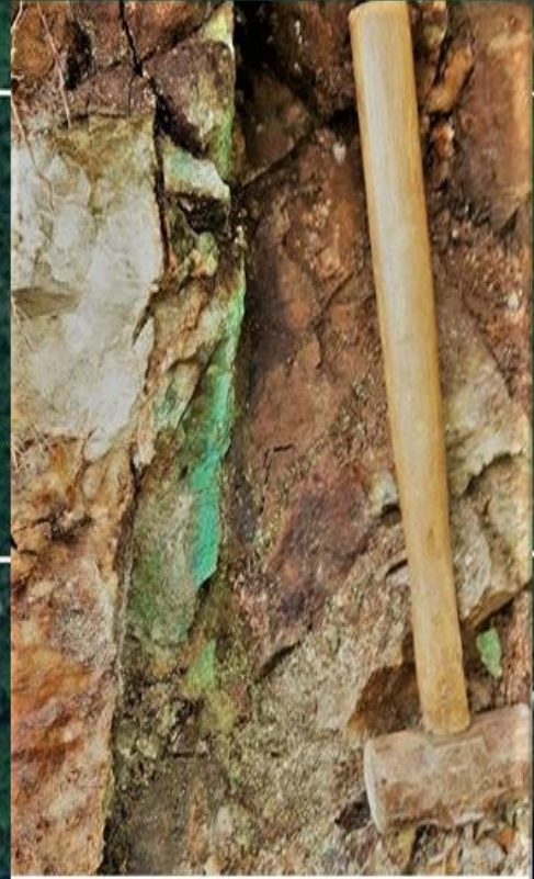
17 U 470115.00 m E 5344251.00 m N Sample 03 Report Number: A18-06714 7.6PPM AG, 3.94% CU, 112PPM ZN,
