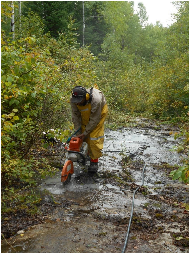
Figure 2. A-Star Prospecting cutting channel samples, Hawkins Property, Sept 7, 2019.
