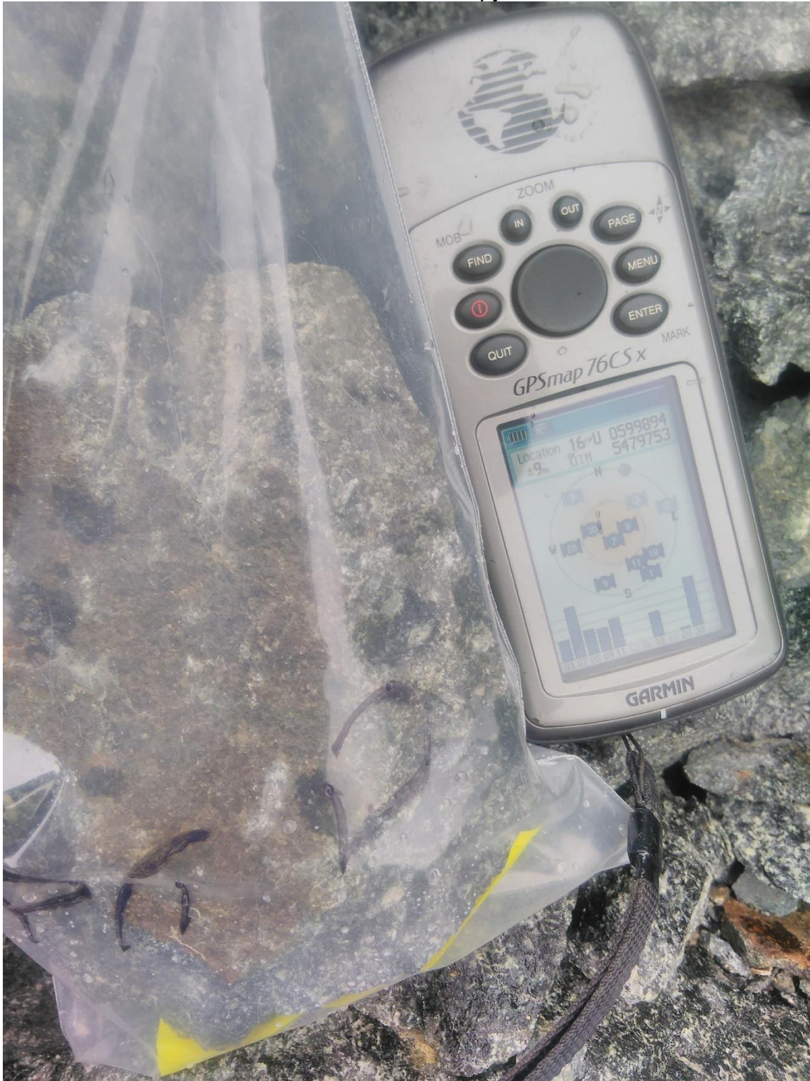
PIT-D: Medium grained mafic dike (diorite-gabbro) with 0.5cm white feldspar in hornblende matrix minor with fine disseminated pyrite.
