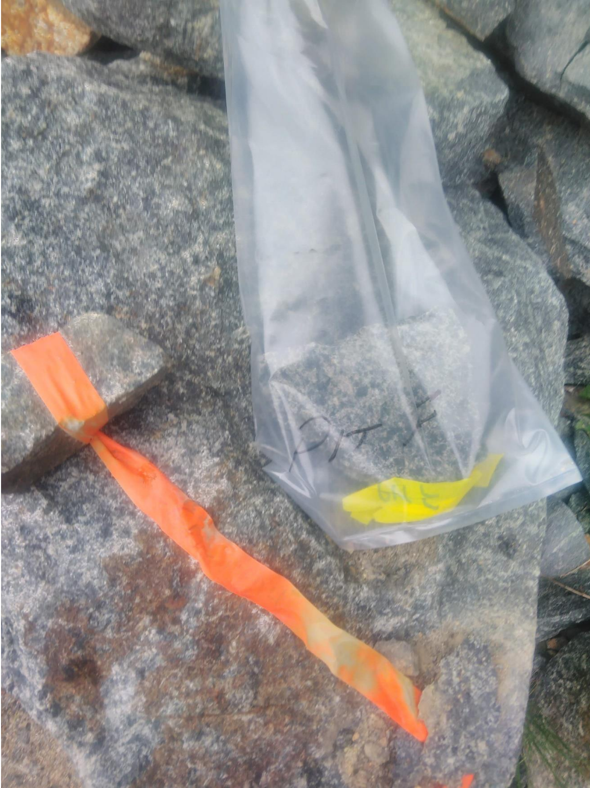
PIT-F: Medium grained mafic dike (diorite-gabbro) with 0.5cm white feldspar in hornblende matrix with minor, fine disseminated pyrite.
