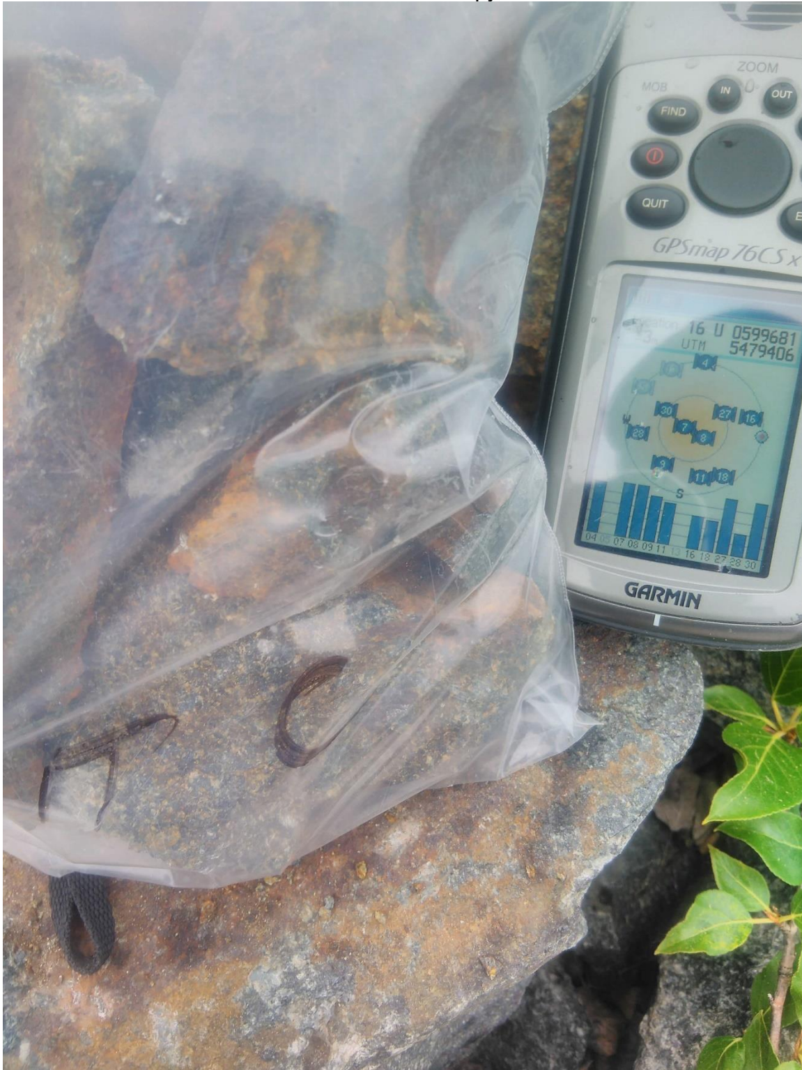
PIT-C: Medium grained mafic dike (diorite-gabbro) with 0.5cm white feldspar in hornblende matrix minor with fine disseminated pyrite.
