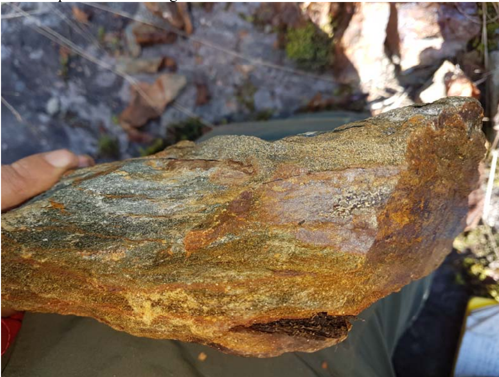
Figure 9. Rusty, sulphidized magnetic iron formation is parallel the 9 Zone quartz veins. Sample returned 1.4 g/t Au.
