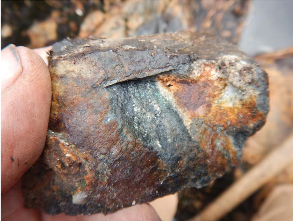
Figure 15. Sulphidized quartz vein with malachite stain at Eagle River (W384) returned 0.16 g/t Au.
