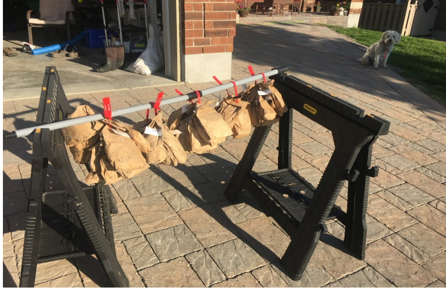
Figure 8: A single line (specifically a L-East that runs north-south, see Fig. 5 for a depiction of the line-grid map) of St. Laurent soil samples drying.
