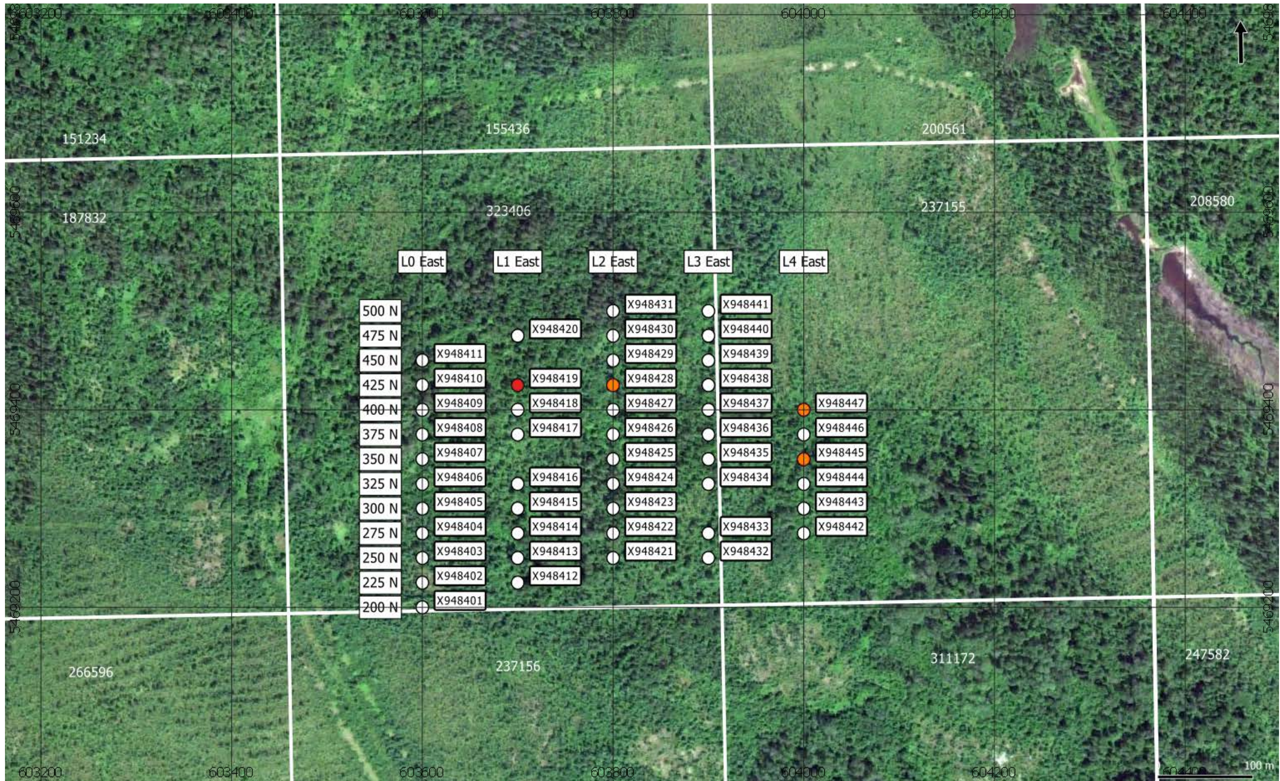
Figure 17: Anomaly map for palladium samples collected for soil geochemical survey on Pancontinental Resources Corporation's St. Laurent property. Soil sample locations are indicated by labelled dots; where orange dots indicate anomalous samples (> 2.2 ppb), red dots indicate far outliers (> 3.8 ppb), and white dots indicate samples that fell below anomaly thresholds (See App. A: Tab. 2 for detailed UTM and grid line coordinates). Claim numbers are indicated by white text and claim boundaries are indicated by white lines.
