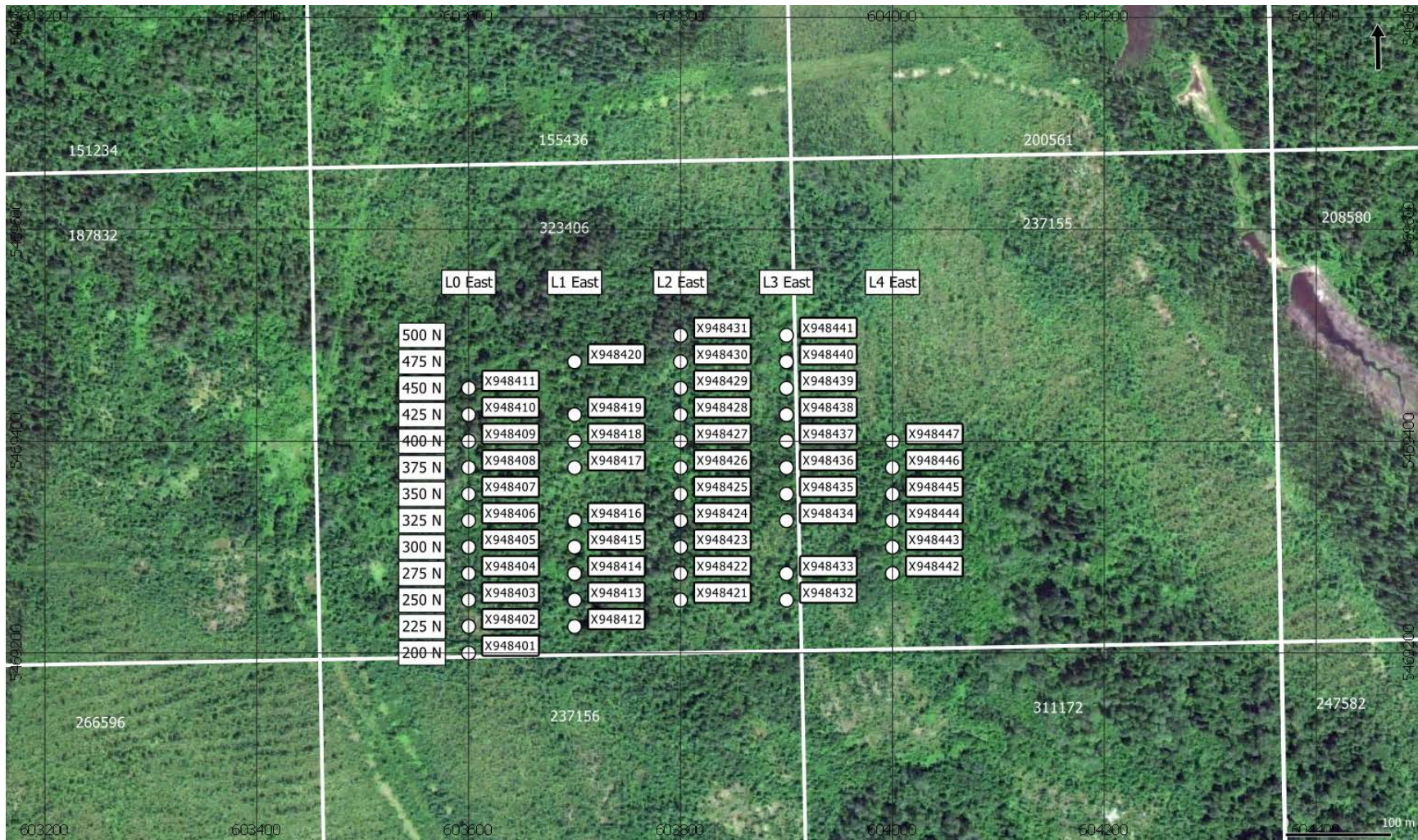
Figure 5: The soil sample line-grid indicating the locations of sample stations where soil samples were collected for soil geochemical survey. Soil sample locations are indicated by white dots (See App. A: Tab. 2 for detailed UTM and grid line coordinates). Claim numbers are indicated by white text and claim boundaries are indicated by white lines.
