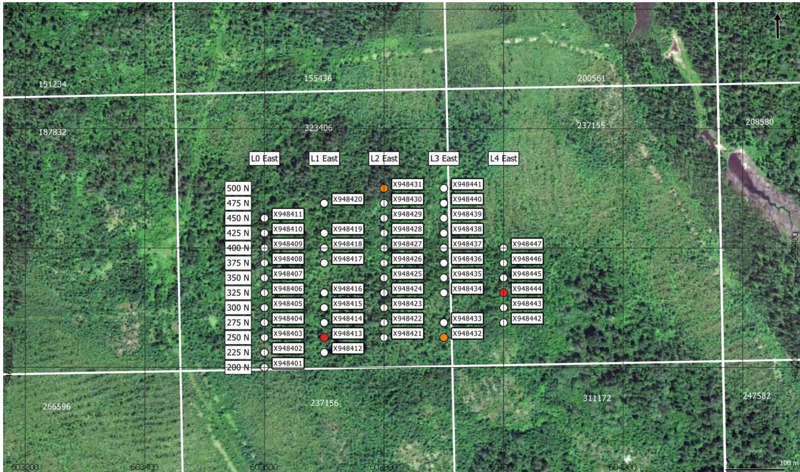
Figure 15: Anomaly map for cobalt samples collected for soil geochemical survey on Pancontinental Resources Corporation's St. Laurent property. Soil sample locations are indicated by labelled dots; where orange dots indicate anomalous samples (> 13.0 ppm), red dots indicate far outliers (> 16.0 ppm), and white dots indicate samples that fell below anomaly thresholds (See App. A: Tab. 2 for detailed UTM and grid line coordinates). Claim numbers are indicated by white text and claim boundaries are indicated by white lines.
