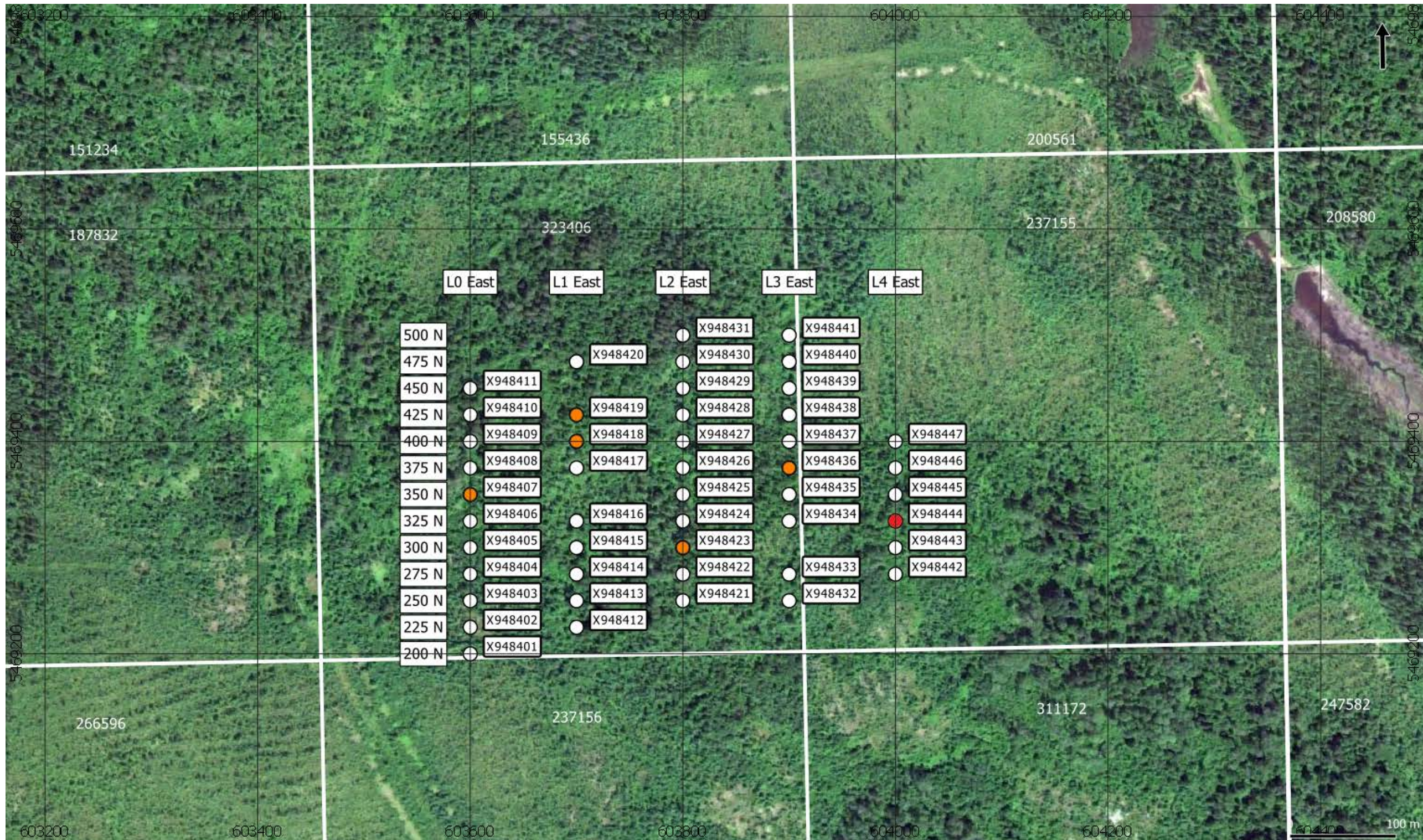
Figure 13: Anomaly map for gold samples collected for soil geochemical survey on Pancontinental Resources Corporation's St. Laurent property. Soil sample locations are indicated by labelled dots; where orange dots indicate anomalous samples (> 1.0 ppb), red dots indicate far outliers (> 1.4 ppb), and white dots indicate samples that fell below anomaly thresholds (See App. A: Tab. 2 for detailed UTM and grid line coordinates). Claim numbers are indicated by white text and claim boundaries are indicated by white lines.
