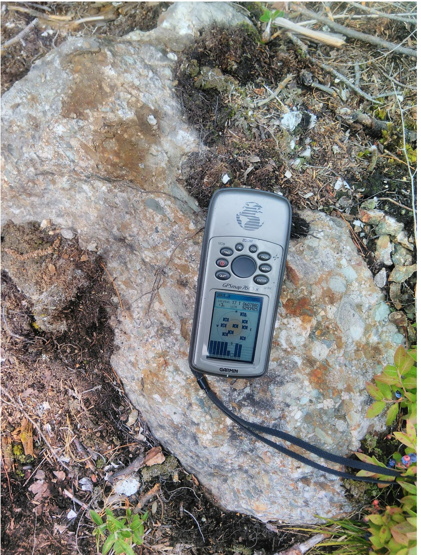
Photo #1 Sample PENSE-2019-01, Coleman member conglomerate. Note the blebby rust spots caused by pyrite. The sample was taken at location NAD83 Zone 17, 607880E, 5293925N. The gold assay returned 0.060 ppm, silver <10ppm and multi element highlights of 14.3 % iron and 5.98% magnesium. The matrix of the conglomerate was highly variable, chaotically sorted, includes irregular to rounded clasts which rarely exceeded 10 centimeters in size. Surprisingly consistent over the entire expanse of the outcropping, void of laminating siltstone layers of veining of any type within. The author will note a similar conglomerate found at the north Silverfields Property in cobalt where it sharply ramps up against the diorite. The outcrop was not prospected to the west where it is in contact with Nipissing diabase sill. On OGS Preliminary Map P1222 denotes the sequence from west to east as quartz diorite (observed), conglomerate (observed), quartzite-arkose (observed), argillite (observed on west side of Pontleroy Creek) and then a sequence of intermixed early Precambrian metasedimentary to mafic intrusive to mafic to ultramafic intrusive rock lithologies (not observed).
