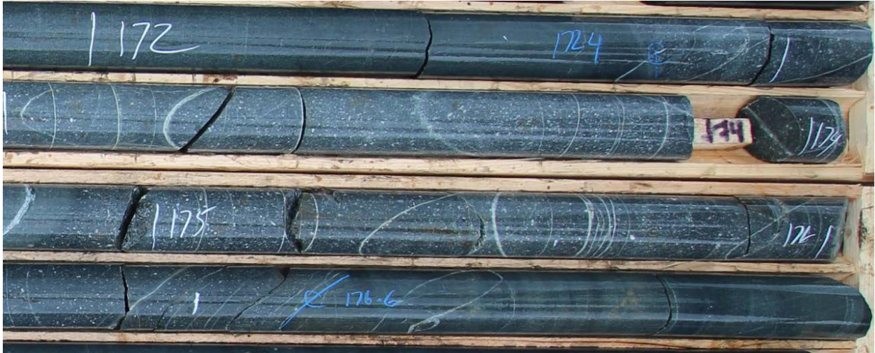
Figure 15: Intermediate Dike (IDIKE) from SL-19-03, approximately 174 m downhole. Sharp upper and lower contact.
