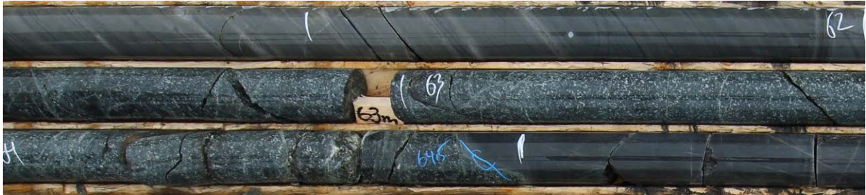
Figure 17: Argillite (ARG) from SL-19-04, approximately 62 m downhole. Top row is argillite with banded/laminated texture.
