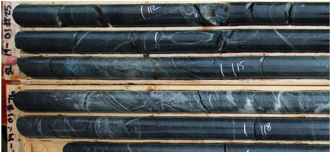
Figure 16: Mafic Volcanic (MVOLC) from SL-19-01, approximately 115 m downhole. Flow breccia and pillow selvages visible.
