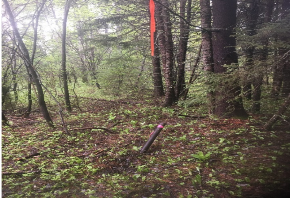
Figure 7: Drill casing from the 1965 R,S.Gray drill program located at UTM: NAD83 17U 603677E 5469253N.
