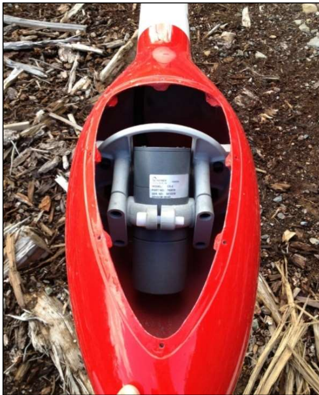
Figure 16: View of cesium vapor magnetometer. Sensor oriented 45° from vertical to couple with local magnetic field at the White Reserve survey block.
