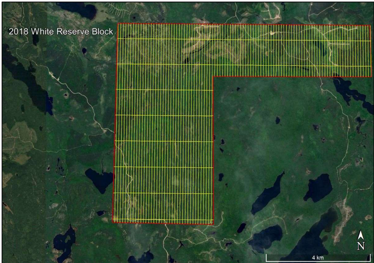
Figure 3: Plan View – 2018 White Reserve survey block boundary in red with actual flight lines in yellow.
