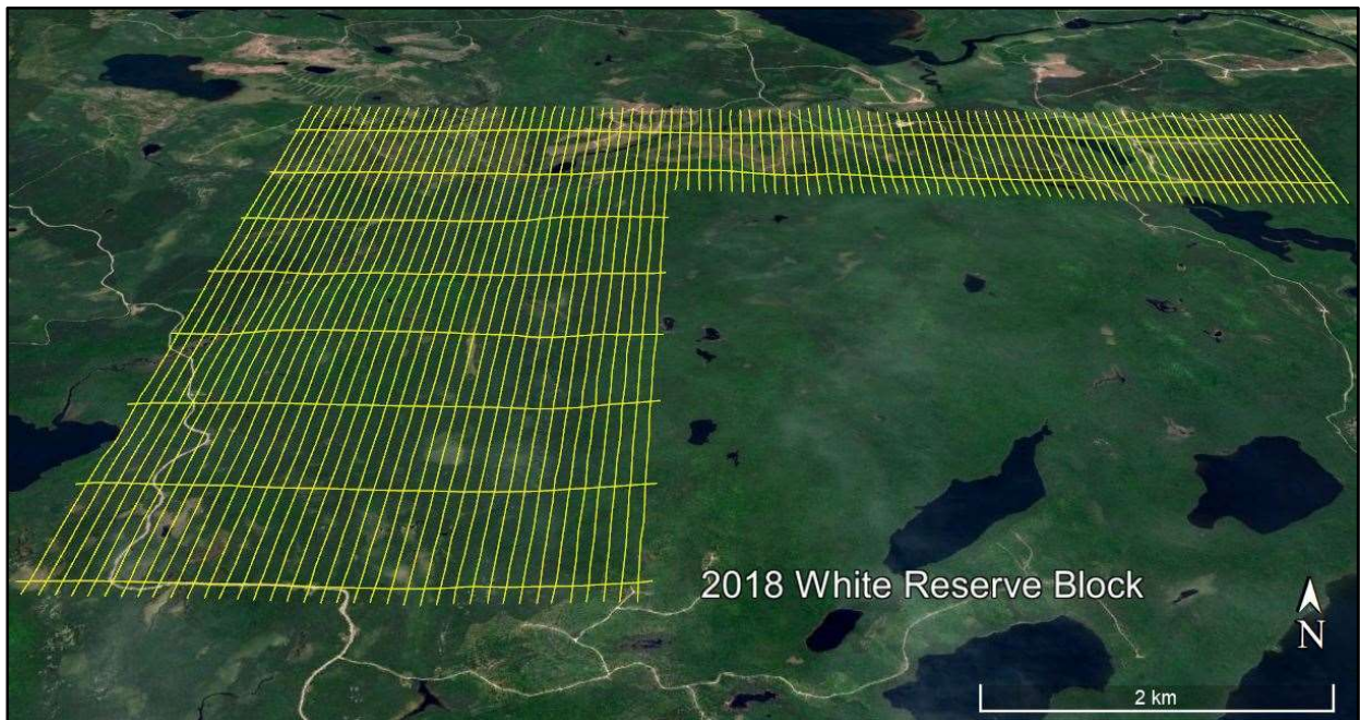
Figure 4: Terrain View – 2018 White Reserve survey block with actual flight lines displayed in yellow.
