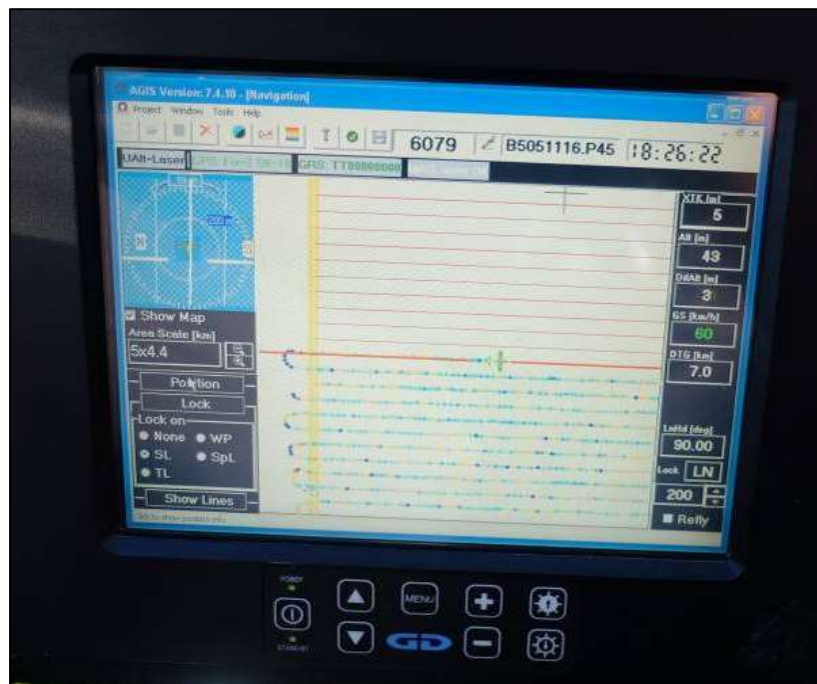
Figure 15: AGIS operator display installed in the Bell 206B Jet Ranger survey helicopter, with screen displaying real time flight line recording and navigation parameters. Additional windows display real time geophysical data to operator.
