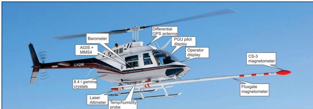
Figure 14: Survey helicopter equipped with geophysical equipment.
