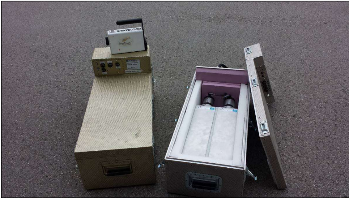
Figure 17: GRS-10 thallium-activated sodium iodide gamma spectrometer crystal packs. The open unit on the right shows two individual 4.2 litre gamma detectors.
