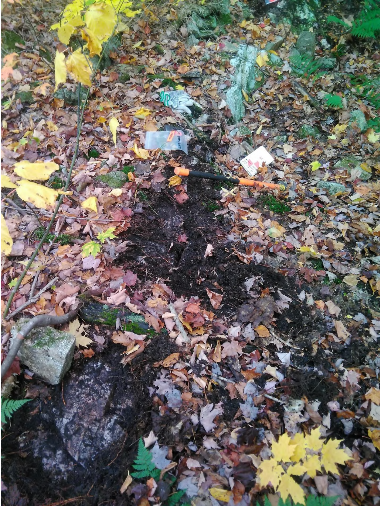
October 10, 2019, new discovery exposed quartz veining, Wells-2019-05, dip 85^{\circ} - 90^{\circ} , strike 80^{\circ} east.
