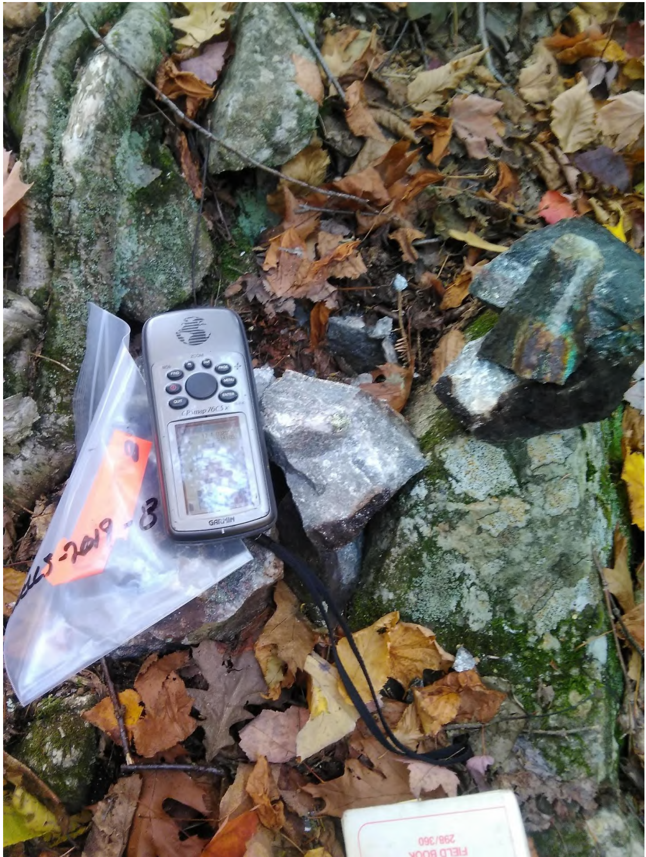
October 10, 2019, sample of Wells-2019-08, quartz vein in shear in diorite, blebs of chalcopyrite.
