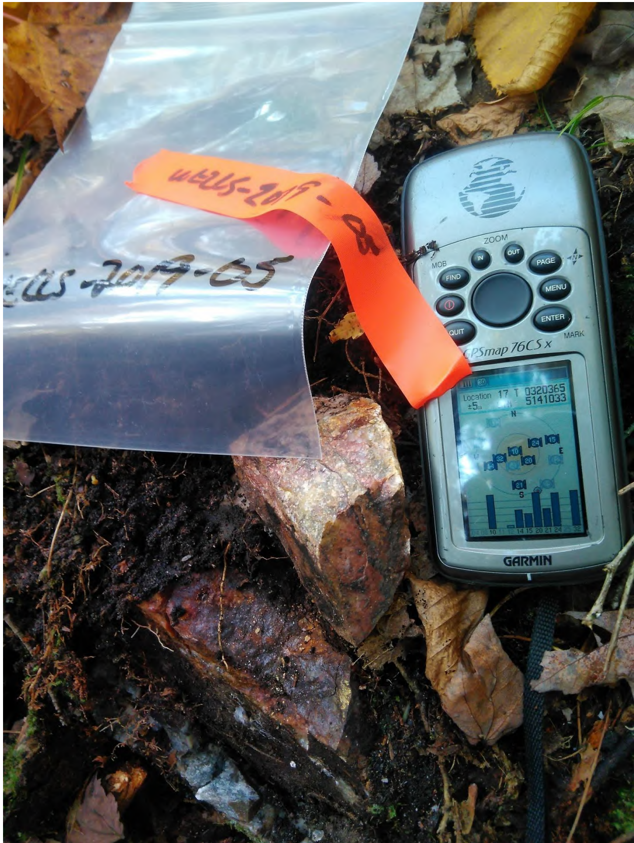
October 10, 2019, new discovery, location of sample Wells-2019-05, quartz veining + cpy-py in diorite.
