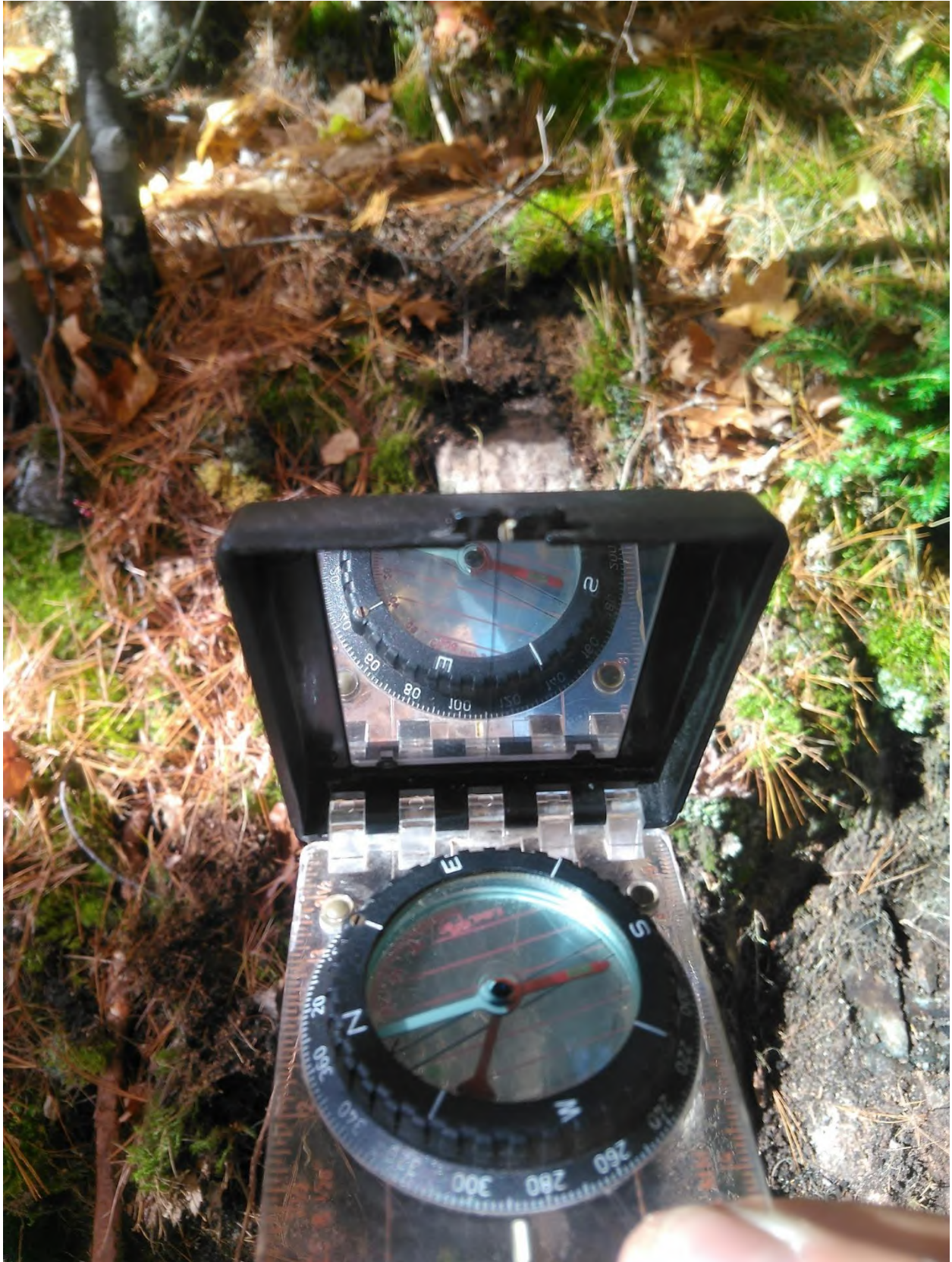
October 10, 2019, quartz vein same as samples 03 & 04 veining is striking 110^{\circ} , 320115\text{E} , 5140370\text{N} .
