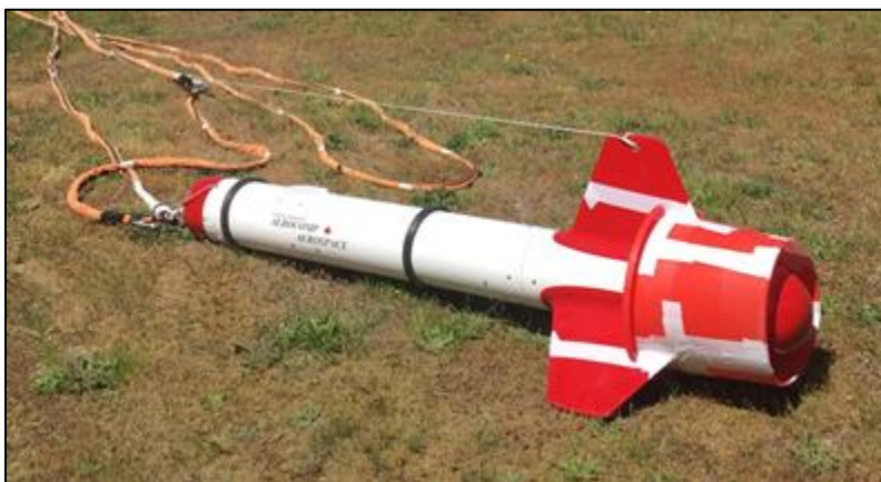
Figure 7 – Airborne magnetometer housing with tow cable.
