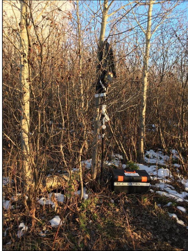
Figure 8 – Base station magnetometer used for diurnal corrections.
