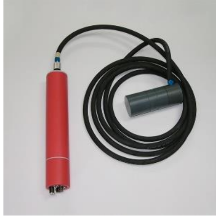
Figure 6 – Scintrex CS-3 magnetometer sensor, cable and electronics.
