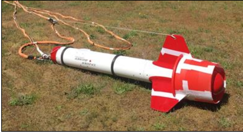
Figure 7 – Airborne magnetometer housing with tow cable.
