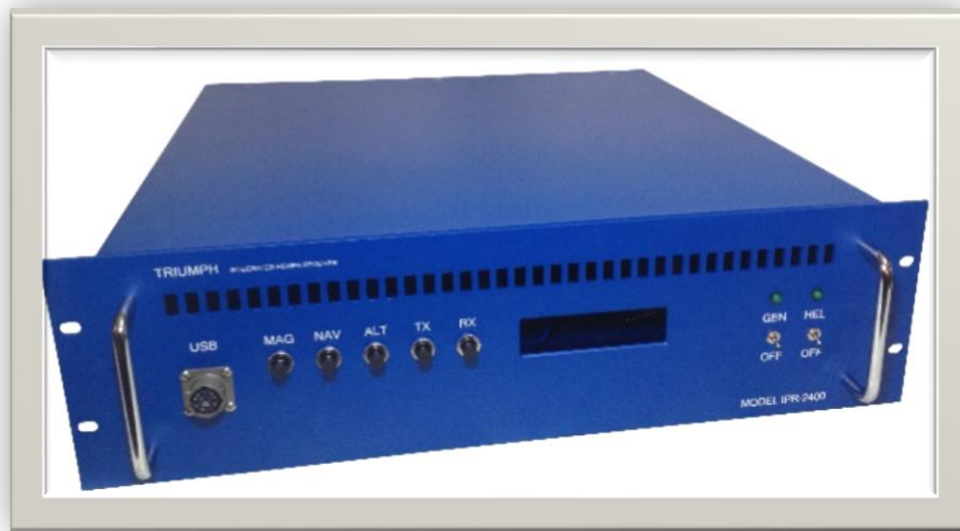
Figure 12 – Triumph TDS-2400 EM console and acquisition system.
