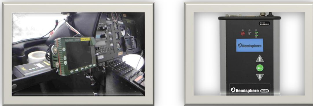
Figure 9 – AgNav main console (left) and Tee-Jet GPS receiver (right).
