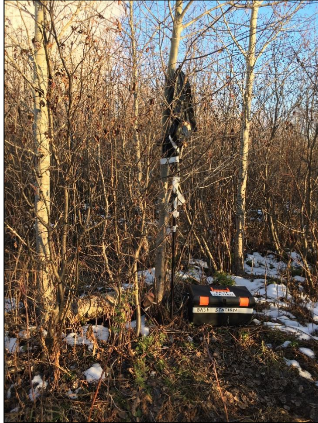
Figure 8 – Base station magnetometer used for diurnal corrections.
