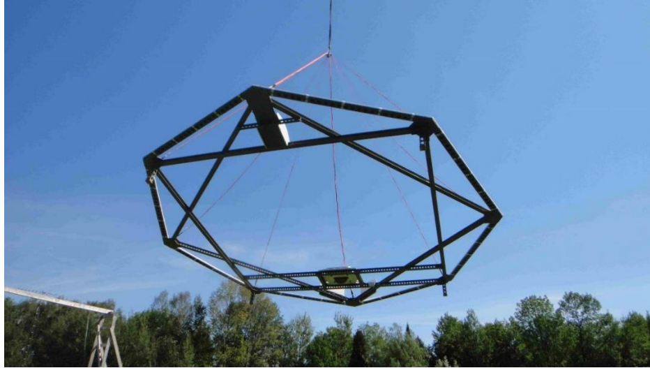
Figure 4 – The Triumph AirTEM™ TS-150 HTEM System.
