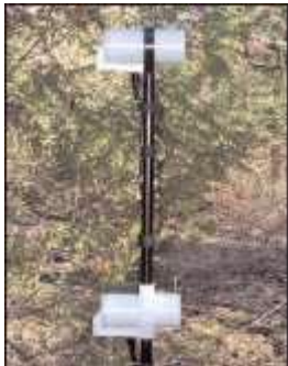
An important GSM-19 design feature is that its gradiometer sensors measure the two magnetic fields concurrently to avoid any temporal variations that could distort gradiometer readings. Other features, such as single-button data recording, are included for operator ease-of-use.
