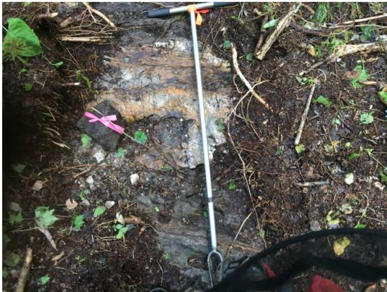
Photo 3 – A 0.70 Meter Wide Rusty Quartz Vein Near Line 2W/ 2N (555373E/ 5511157N)
