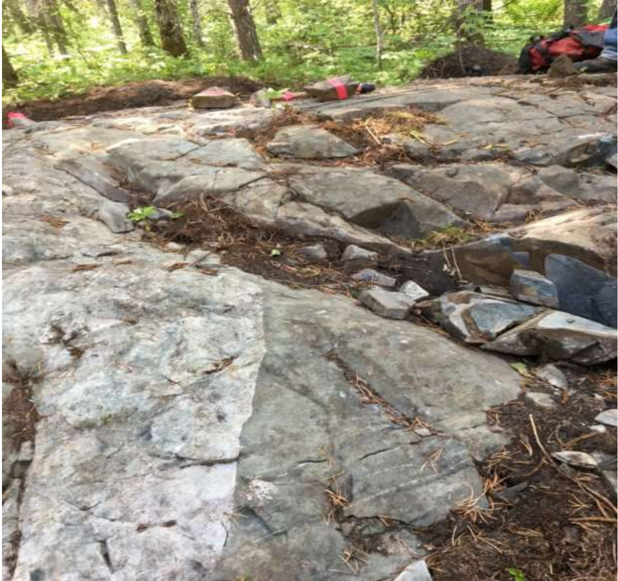
Photo 5 – Mafic to Intermediate Metavolcanic at 160^{\circ} Trending Contact. Historic Grab Samples G29353 and G29354 in Narrow Quartz Vein at Top of Photo at 555090E/ 5511084N
