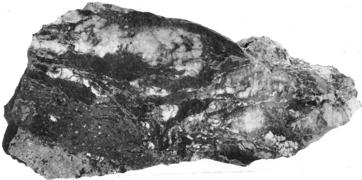
Polished specimen of ore from McMillan mine. Argillite and chlorite (black) with quartz (white), pyrrhotite (dark-grey), and arsenopyrite (light-grey).
