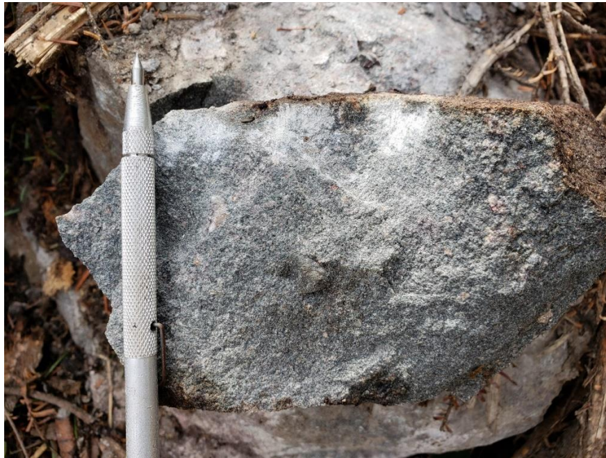
Figure 23: Sandstone (Lorrain(?))- Medium grey to pink, fine to medium grained sand, massive to very weakly foliated (laminated?), well sorted. Locally minor biotite formation, and pink hematite(?) staining.
