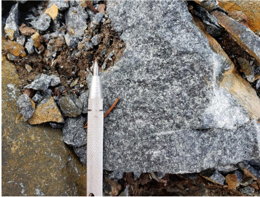
Figure 22: Diabase (Nipissing)- medium to dark green grey, medium grained, massive, predominantly equigranular with local coarse grained patches, weakly to moderately magnetic; Weak chlorite alteration and weak sericite alteration of plagioclase; trace fine grained pyrite. (Figures 22, 23, 24, all taken traverse date September 27, 2018)
