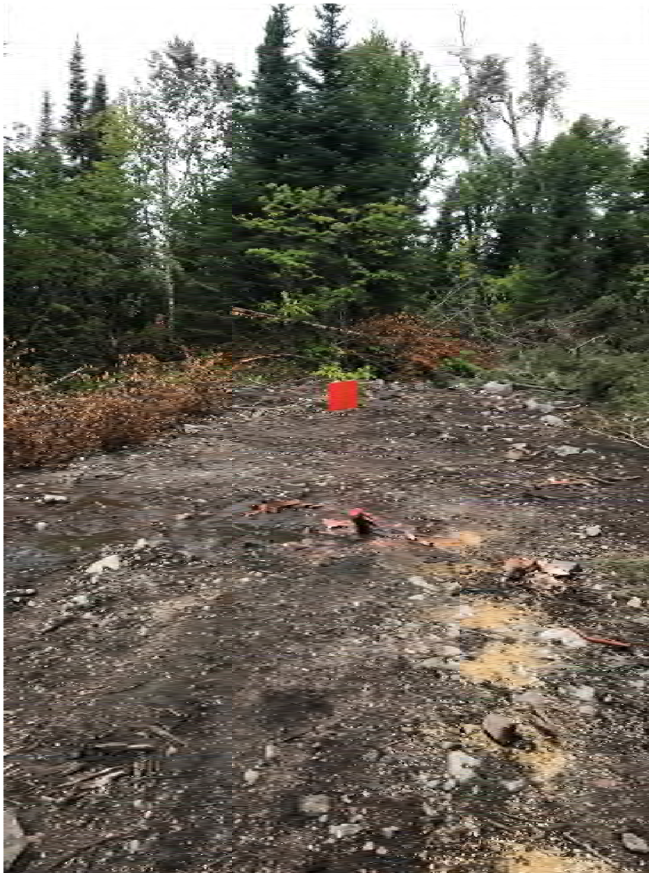
Figure 6: Example of Casing Cap and Flag at JF-18-02 Drill Site.
