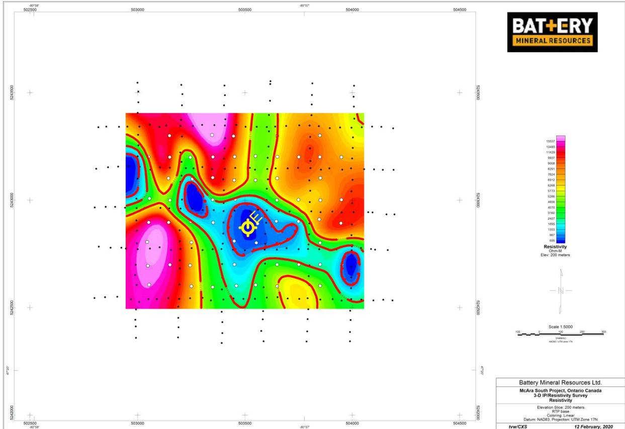
Figure 28 – The 200 meter resistivity Elevation slice used to pick Rho Target E.
