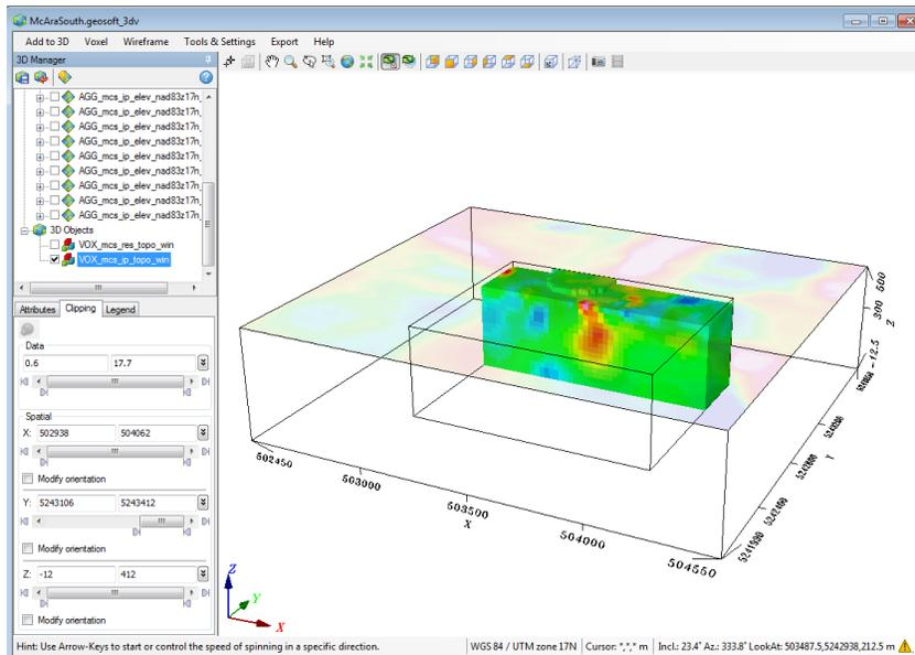
Figure 12 – The 3-D IP voxel clipped (Y coordinate) in section view at the north edge of the model. Note the IP response at the northern edge of the voxel tends to be shallower and depth extent limited.
