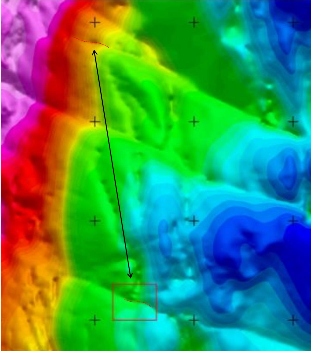
Figure 3 – An enlargement of Figure 2 (1vi image) showing the location of both the McAra and McAra South areas. The red dashed lines show bends in the WNW striking diabase dikes/structures which are interpreted to result in dilation and open space. This open space may host cobalt mineralization.
