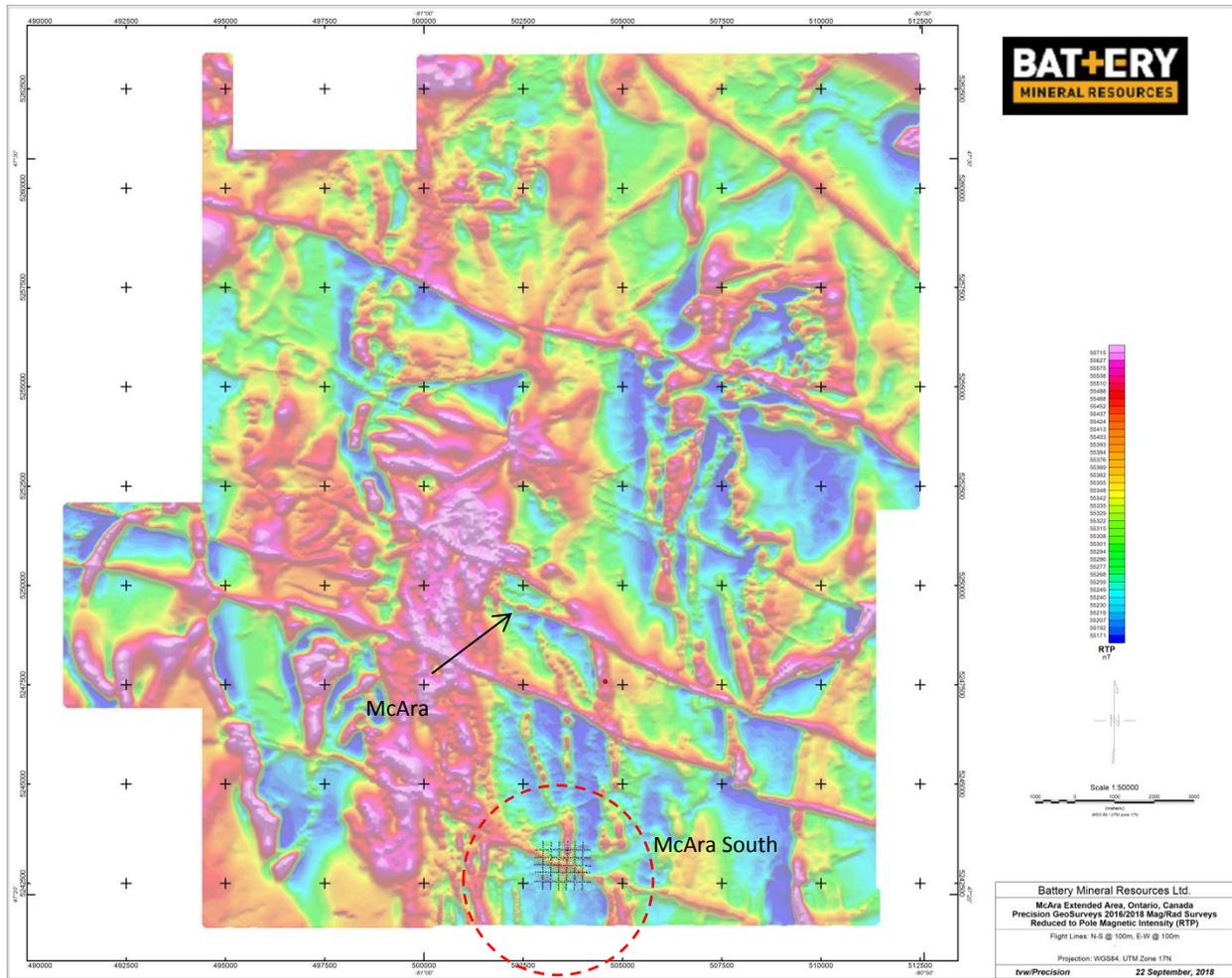
Figure 1 – The location of McAra South prospect (red dashed circle) plotted on the 2016-2018 McAra regional helicopter magnetic (RTP) image. The black arrow points towards the main McAra prospect. Note that NW and NS striking linear magnetic highs (dikes) connect the two prospect areas.
