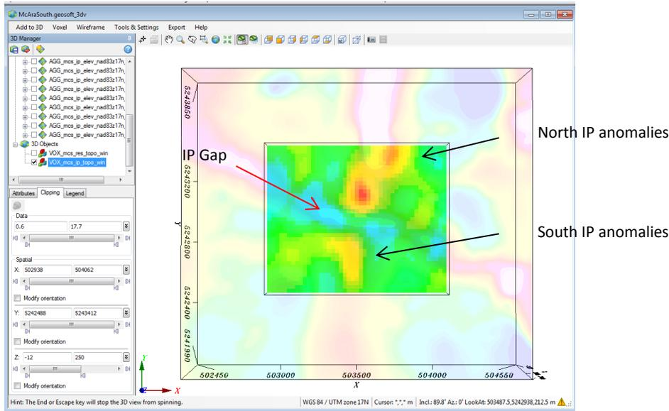
Figure 9 – The 3-D IP voxel clipped at Z equals 250 meters elevation. Note the northern IP anomalies are getting larger and still occur along the edges of the NS striking Nipissing diabase intrusive. The southern IP anomaly is starting to be visible and also occurs along the edge of the NS striking Nipissing diabase intrusive. Note there is a gap in the IP response where the WNW striking diabase dike/structure cuts through the Nipissing intrusive.
