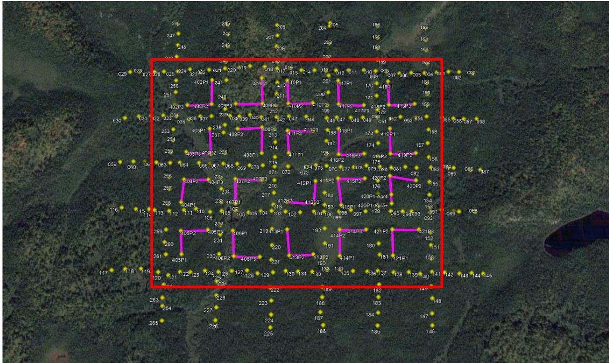
Figure 4 – The CXS 3-D IP/resistivity array used at the McAra South prospect area. The yellow dots are current injection points. The purple elbows show the receiver arrays. The red polygon indicates the portion of the 3-D array where the inversion model is used for interpretation in this report.
