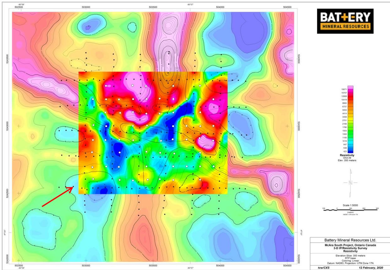
Figure 23 – The shallow 350 meter resistivity elevation slice plotted on the RTP magnetic base map. Note the magnetic contours show up through both data sets for anomaly location purposes. The red arrow indicates the location of the NE-SW near surface resistivity low.
