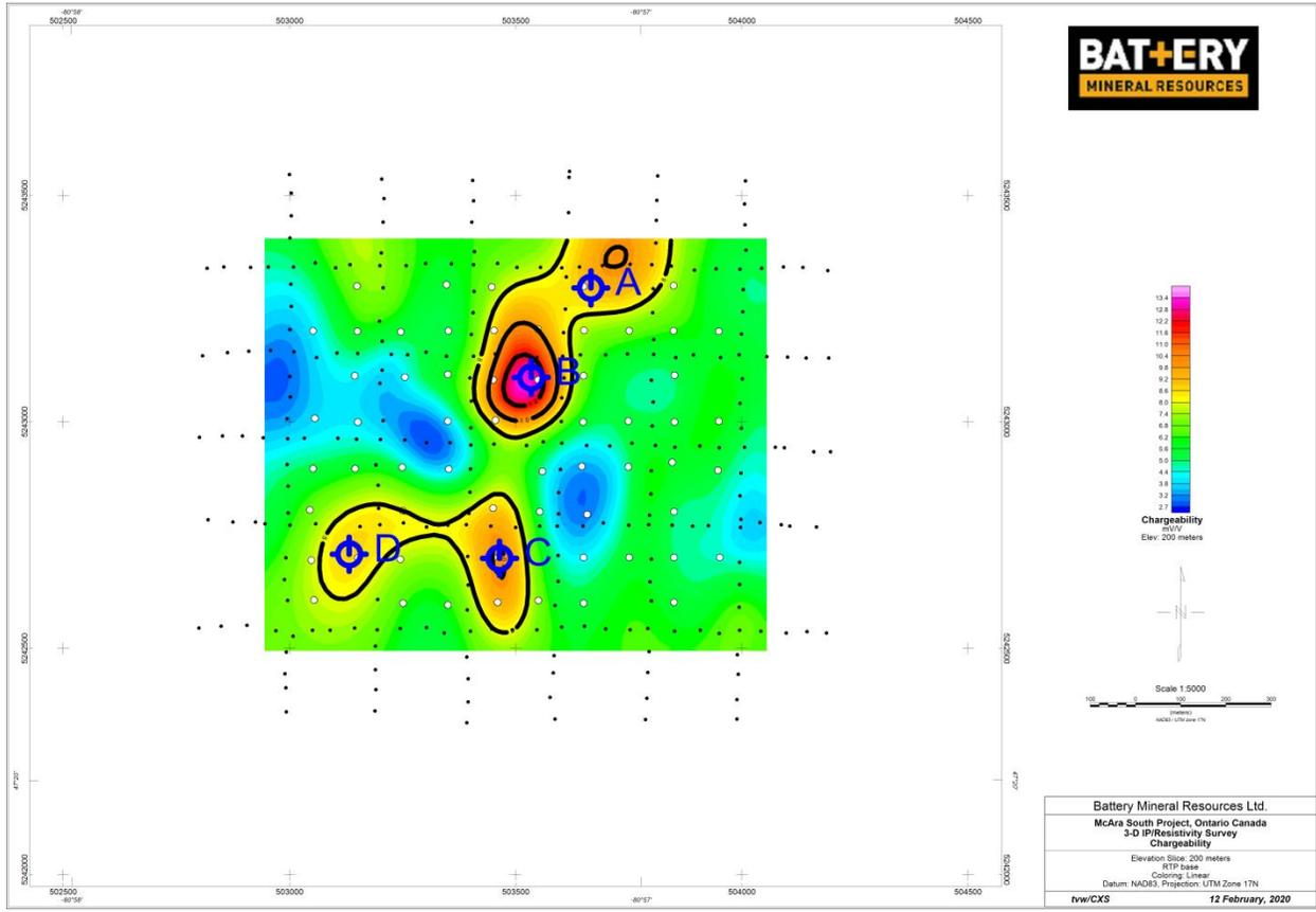
Figure 26 – The 200 meter IP elevation slice used to pick IP Target C.
