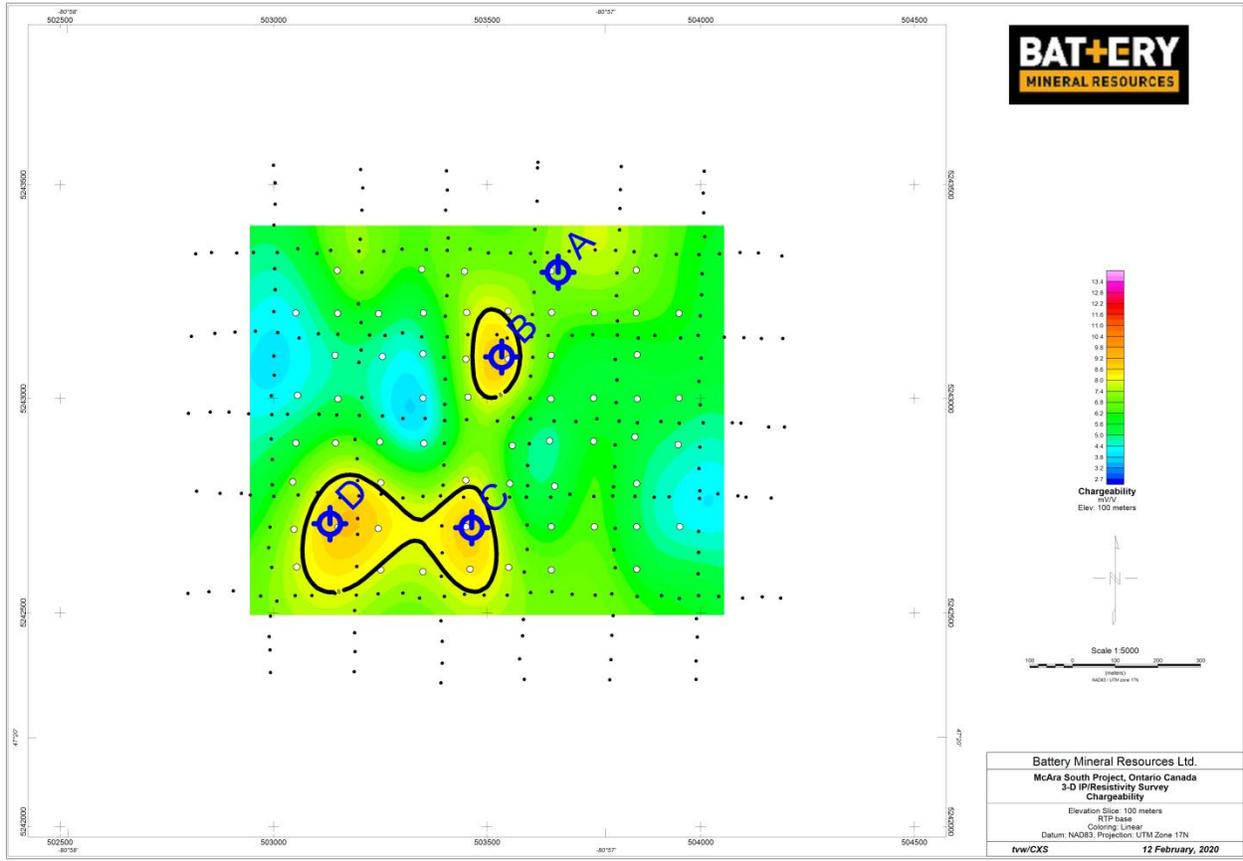
Figure 27 – The 100 meter IP elevation slice used to pick IP Target D
