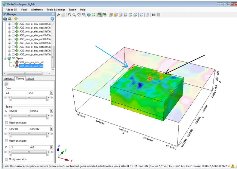
Figure 7 – The unclipped IP voxel viewed down and to NW. Note the two small IP highs (hot colors) in the center/north area of the block (black arrow). These IP responses occur at the edges of the Nipissing intrusive. A third small IP anomaly occurs at the NW corner of the block. It is located along the edge of the WNW striking diabase dike (blue arrow).
