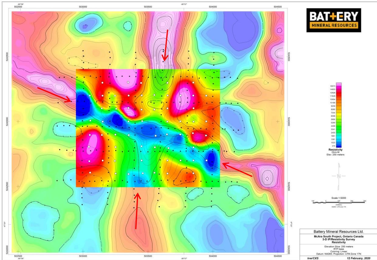
Figure 24 – The deeper 250 meter resistivity elevation slice plotted on the RTP magnetic base map. Note the magnetic contours show up through both data sets for anomaly location purposes. The shallow NE-SW near surface resistivity low is gone. The deeper WNW and N-S intrusive resistivity lows show up clearly at this elevation (red arrows).
