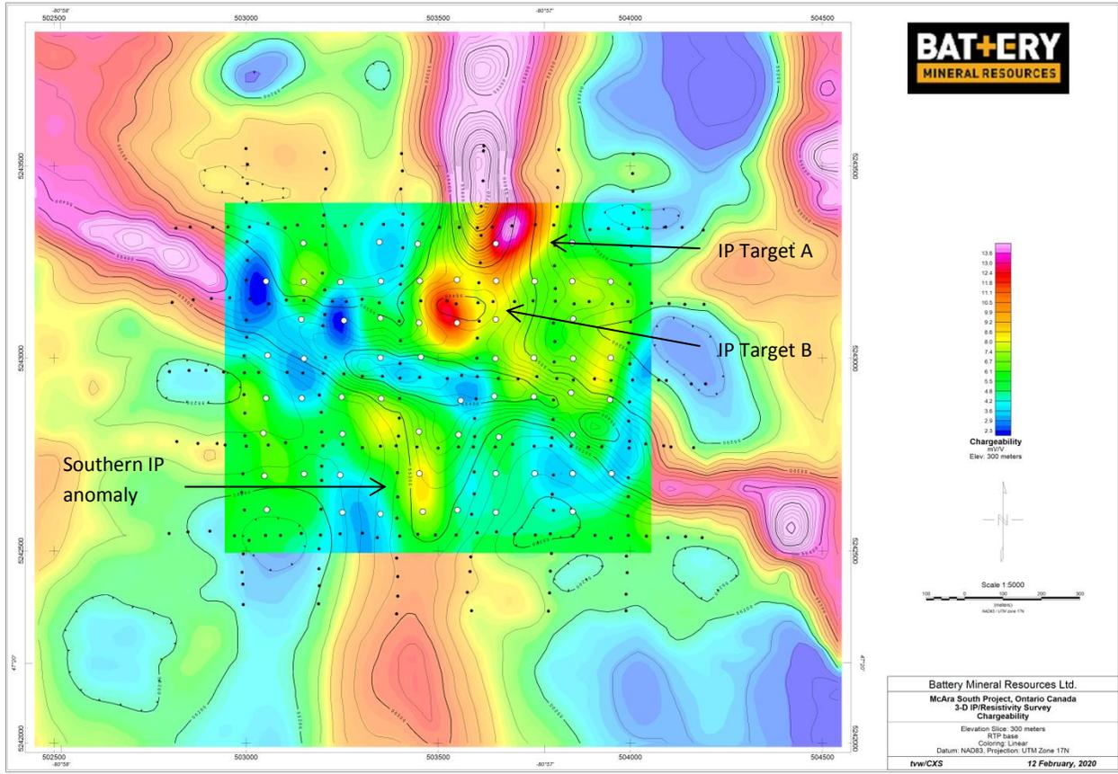
Figure 16 – The 300 meter elevation IP slice plotted on the RTP magnetic image. The northern IP anomalies are getting larger. A weak southern IP anomaly is visible at this elevation.
