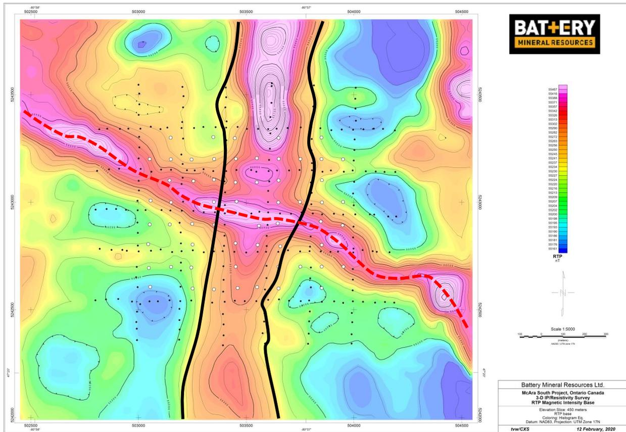
Figure 6 – The detailed helicopter magnetic (RTP) image covering the McAra South prospect. The black lines outline the interpreted N-S striking Nipissing diabase intrusive. The red dashed line highlights the axis of the younger (?) WNW striking diabase dike/structure. Note the 3-D IP/resistivity electrode array is centered on the intersection of these two intrusives.
