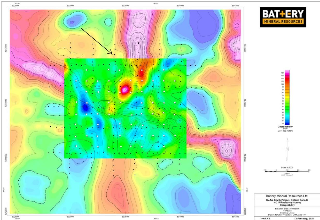
Figure 15 – The 350 meter IP elevation slice plotted on the RTP magnetic image. The shallow IP response in the magnetic low (black arrow) is gone. Two anomalous IP responses occur along the edge of the northern Nipissing diabase intrusive. Note that the magnetic contours show through the IP image. This allows the reader to see how the anomalous IP responses are located with the respect to the magnetic data.
