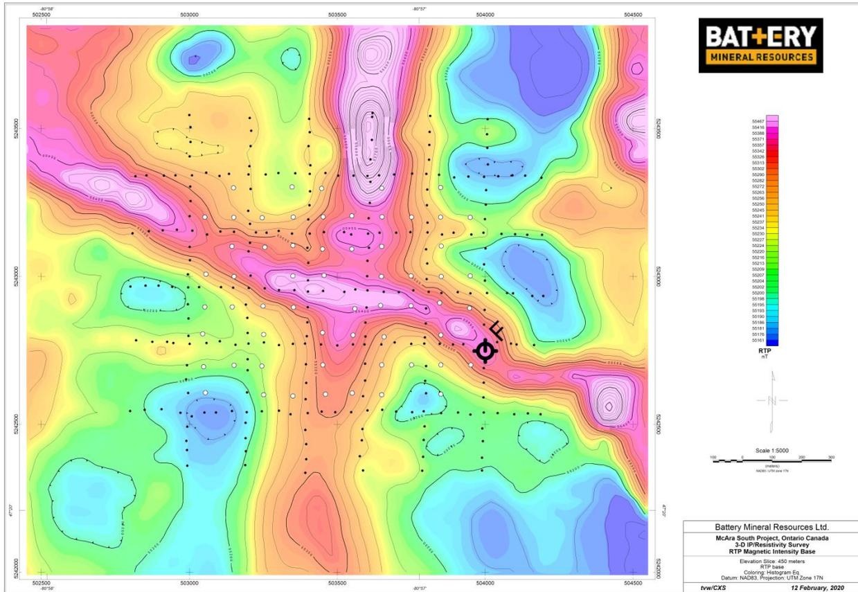
Figure 29– The RTP magnetic image used to pick Mag Target F which is a dilation space opening target based on right lateral strike slip motion along the WNW striking diabase dike/structure. Note there are a series of weak E-W striking dike features mentioned in the report above which might be considered drill targets. I have not selected them here but if they are of geologic interest they should be considered.
