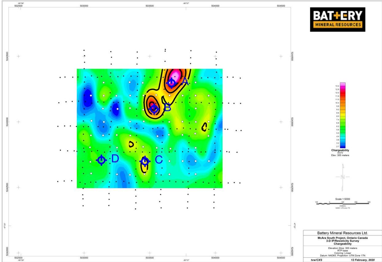
Figure 25 – The 300 meter IP elevation slice used to pick IP Targets A and B.
