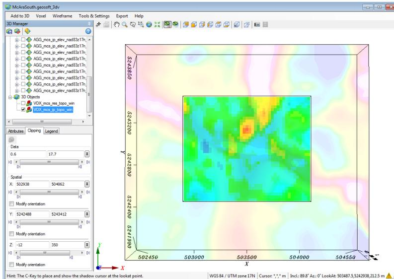
Figure 8 – The 3-D IP voxel clipped at Z equals 350 meters elevation. The magnetic RTP image is faded so that the voxel can be viewed through it. The shallow IP responses occur to the north along the edges of the Nipissing diabase body.
