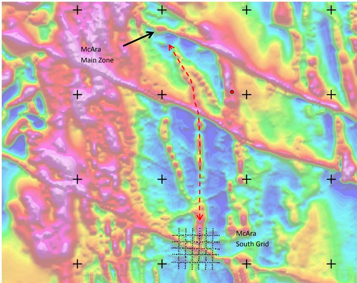
Figure 5 – An enlargement of the McAra regional helicopter magnetic (RTP) data set with the McAra South CXS 3-D IP/resistivity grid plotted on top. Note McAra South occurs at the intersection of a WNW dike/structure and a N-S Nipissing intrusive dike/sill. The dashed red double arrow shows that there is an intrusive connection between the McAra and McAra South prospect areas.
