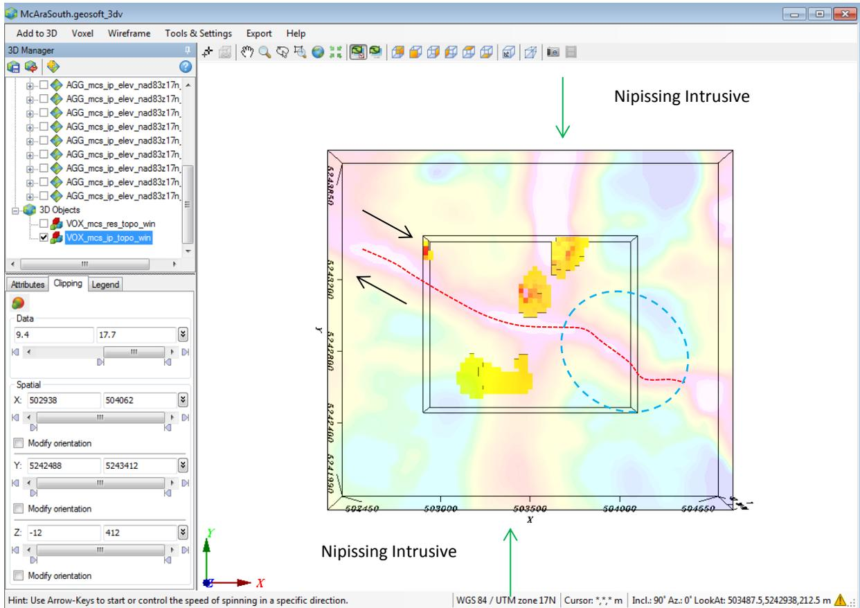
Figure 13 – The 3-D IP voxel clipped to show chargeability values between 9.4 and 17.7 mV/V. Note the close relationship between the IP response and the edges of the interpreted Nipissing diabase intrusion. The red dashed line shows the axis of the WNW striking diabase dike/structure. The blue ellipse indicates an area where the space may be opened if right lateral strike slip motion occurs along the WNW striking structure.
