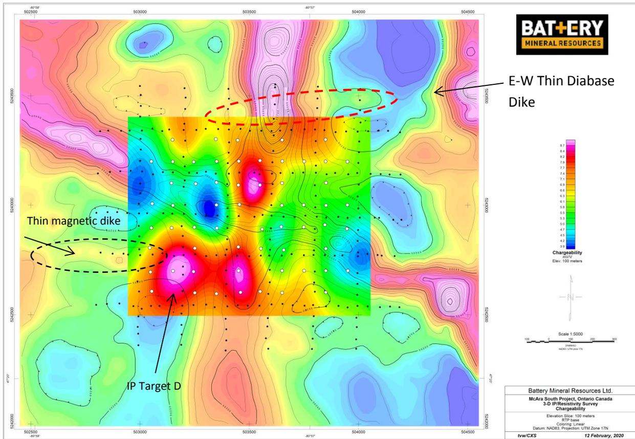
Figure 18 – The 100 meter IP elevation slice cut from the 3-D IP voxel model. The southern anomalies grow with depth and the northern anomalies weaken. The deep target, IP Target D, is identified on the 100 meter elevation slice. This target is estimated to be 250 to 300 meters deep.
