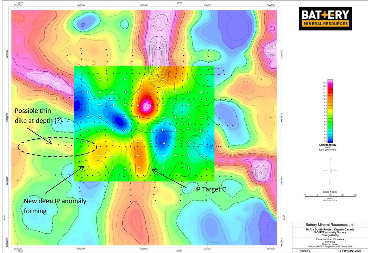
Figure 17 – The 200 meter IP elevation slice cut from the 3-D IP voxel model. The northern IP anomaly on the east side of the Nipissing diabase intrusive continues to weaken at depth. The central and southern anomalies are strengthening and broadening. This 200 meter elevation slice is where the IP Target C is identified. Note a deeper IP anomaly is starting to appear in the SW corner of the grid. It is associated with a thin E-W striking magnetic high interpreted to be a diabase dike.
