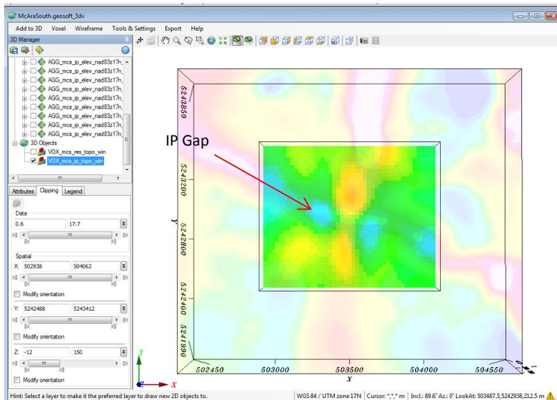
Figure 10 – The 3-D IP voxel clipped at Z equals 150 meters elevation.
