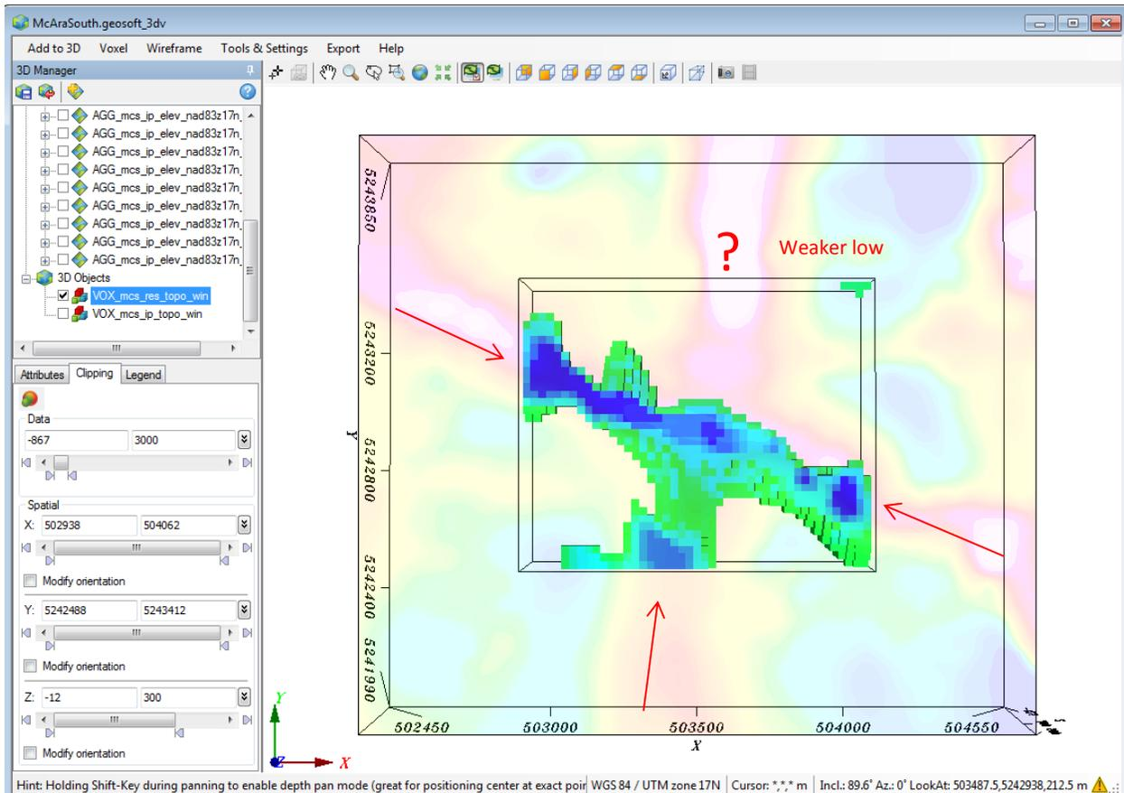
Figure 22 – The 3-D resistivity voxel clipped at 300 meters elevation and at 3000 ohm-m.
