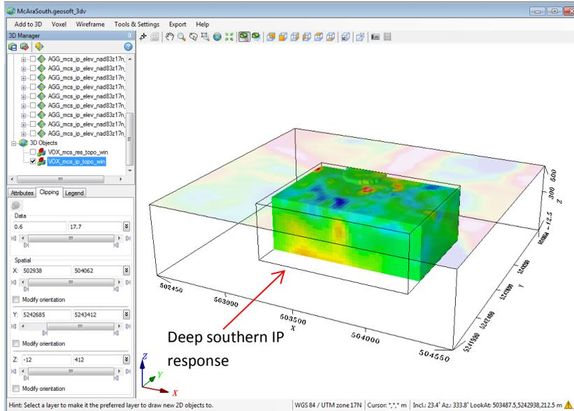
Figure 11 – The 3-D IP voxel clipped (Y coordinate) in section view at the south edge of the model. Note deep IP response at the southern edge of the voxel model.
