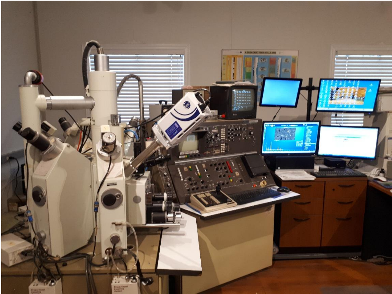
Figure 5. JEOL JXA-733 Superprobe equipped with 5 wavelength spectrometers and an Oxford Instruments Xact Energy Dispersive System housed at the laboratory of Renaud Geological Consulting Ltd.
