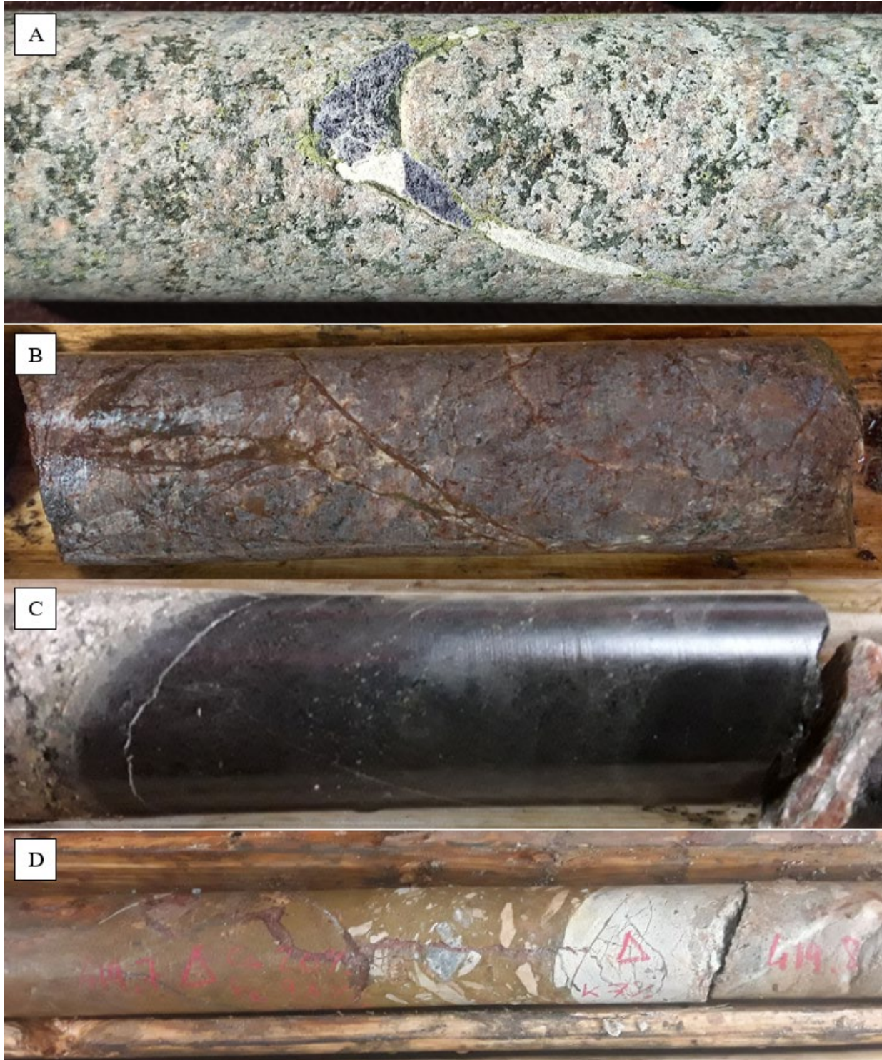
Figure 6: Core photos from Ranoke 2019-2020 drill program. A) Fluorite-calcite-epidote veinlet cutting across foliated Archean granodiorite at 378m in RK20-003; indicates high temperature hydrothermal fluids commonly found within and around IOCG and carbonatite deposits. B) specular hematite veining with potassium-rich halos at 210m in RK19-001a near Archean unconformity; further evidence for IOCG potential. C) least altered, narrow alkalic lamprophyre dyke at 345m in RK19-001b with carbonate amygdales and phlogopite lathe phenocrysts. D) Iron carbonate cemented hydrothermal breccia with rip-up clasts and intense high-K sericite altered lamprophyre wall-rock at 419m in RK19-001b.
