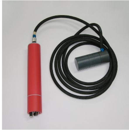
Figure 6 – Scintrex CS-3 magnetometer sensor, cable and electronics.
