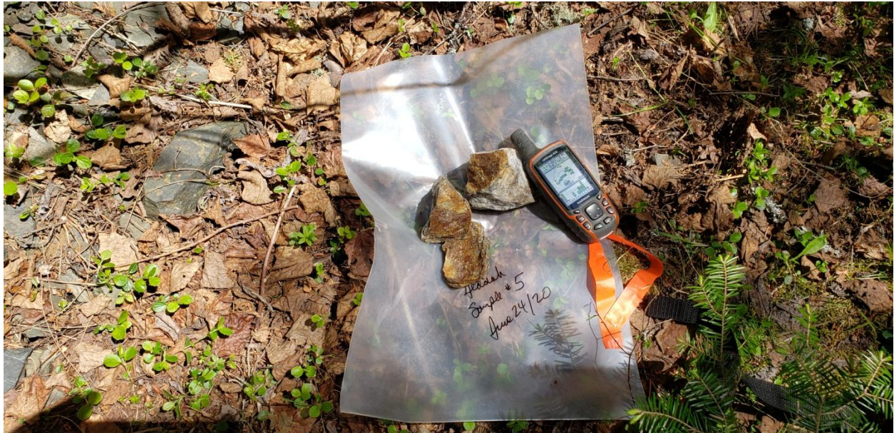
Sample # 5 (tag # 203805) was a grab sample pulled from muck located at 0488309, 5407176. Lab results: 23.4 g/mt Au.
