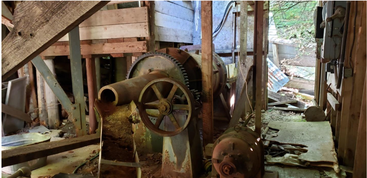
Ball mill in the foreground; grinder and grinder hopper at the rear.
