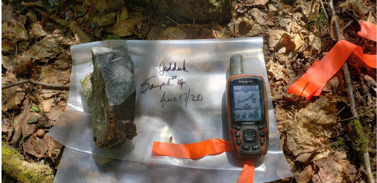
Sample # 4 (tag # 203804) was also retrieved further along the muck pile at 0488240, 5407095. The sample was fine-grained rock with pyrite. Lab results: 3.0 g/mt Au.
