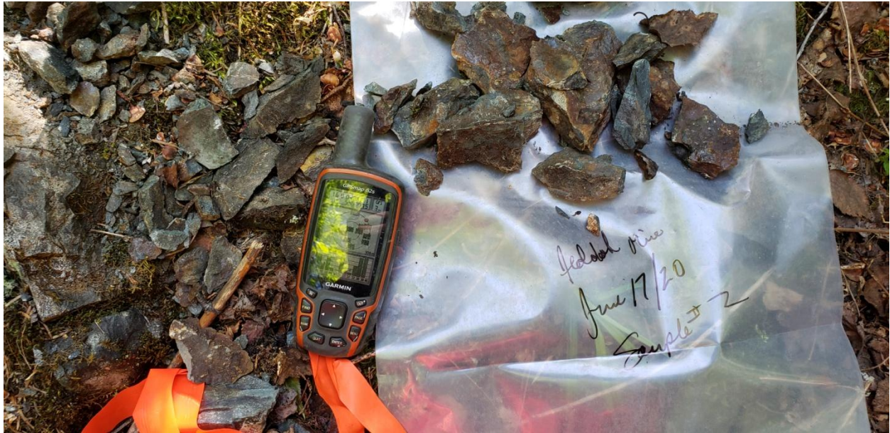
Sample 2 (tag # 203802) which was rusty and showing pyrite, was taken from 0488213, 5407076. Lab results: 0.02 g/mt Au.
