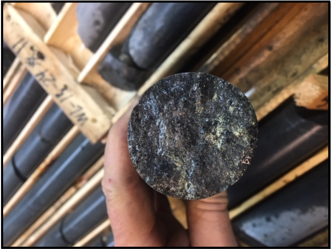
Photograph 4.2.3.2. Pyrrhotite, pyrite and chalcopyrite 49.7m in WL-2018-024.
