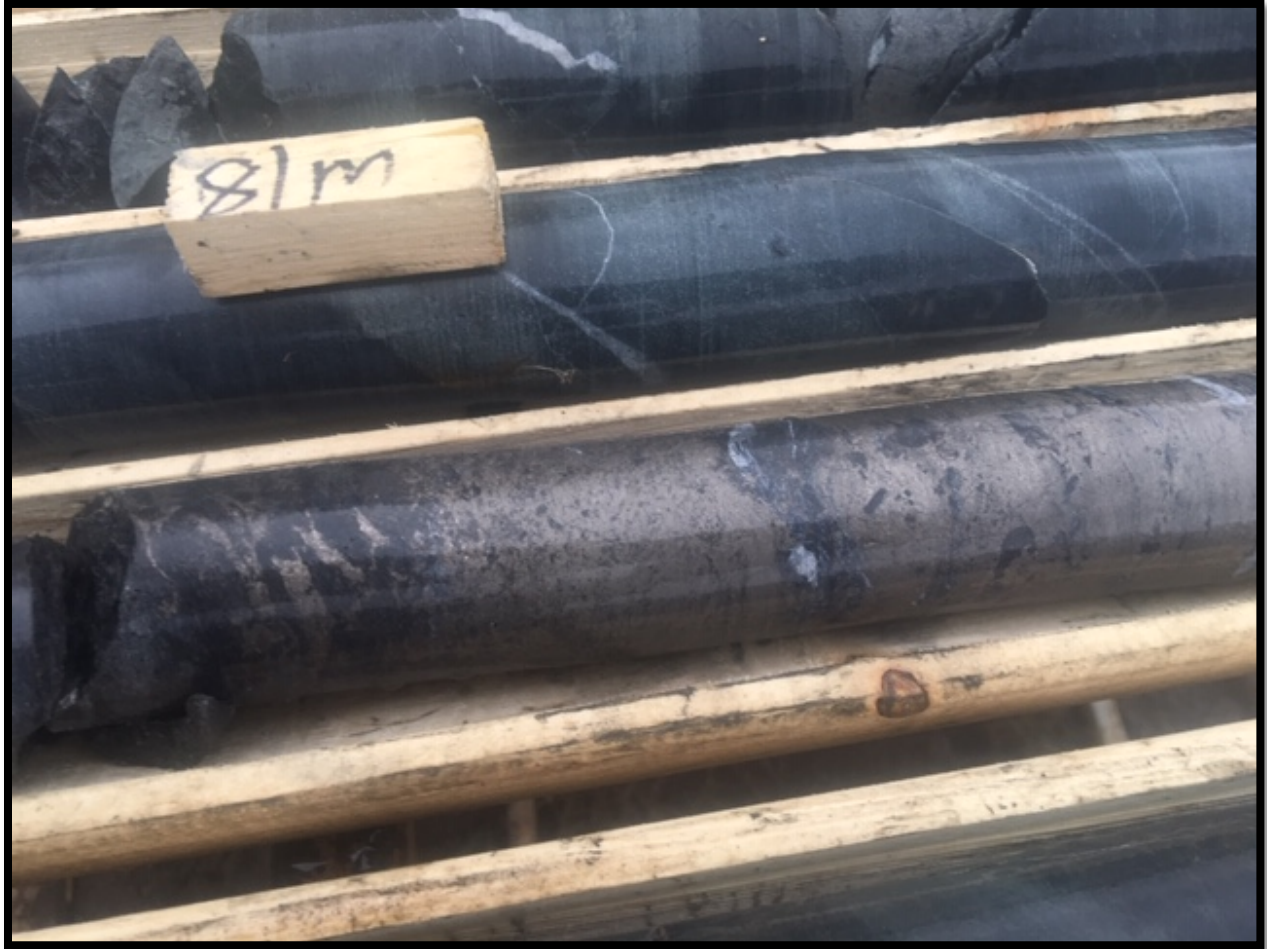
Photograph 4.2.4.3 Details of massive pyrrhotite at 81.0m in WL-2018-25.
