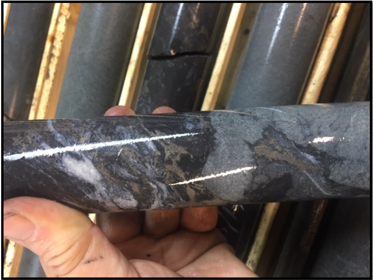
Photograph 4.2.3.1 Iron Formation contact with pyrrhotite and pyrite, WL-2018-024.
