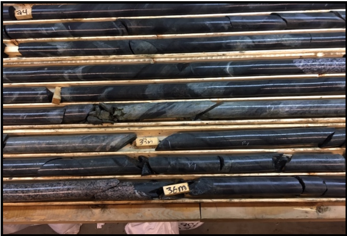
Photograph 4.2.1.3 Quartz veins and alteration, second mineralized zone Kakeeway showing.
