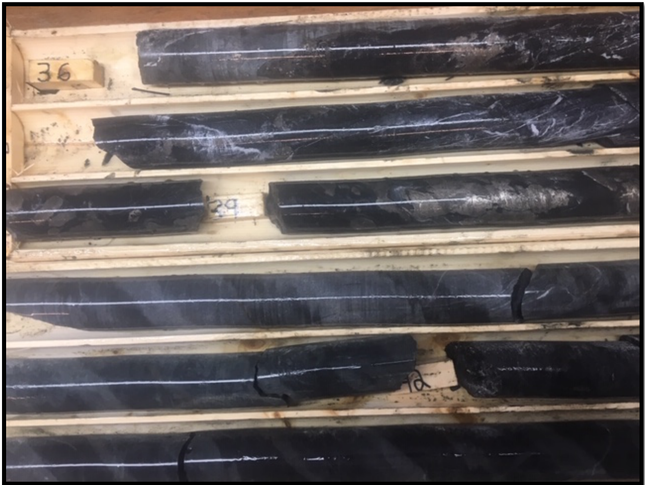
Photograph 4.2.4.1 Pyrrhotite – pyrite mineralized zone 30.7m to 39.7m in WL-2018-025.
