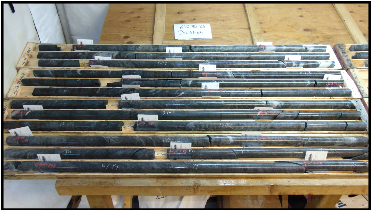
Photograph 4.2.5.4 Silicified and mineralized section 261.31m-to-280.75m drill-hole WL-2018-026.
