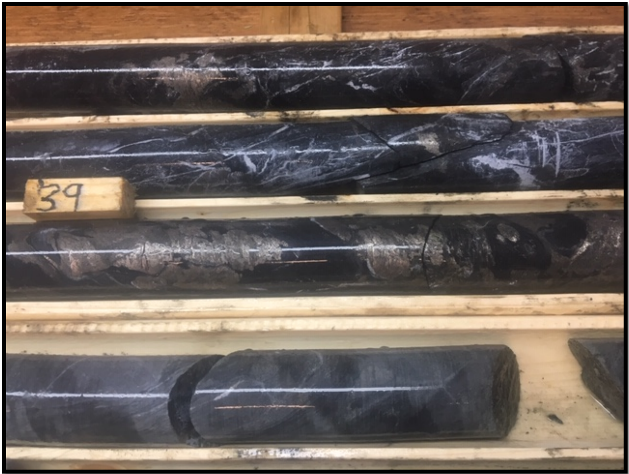
Photograph 4.2.4.2 Details of mineralization 39.0m – 39.7m in WL-2108-025.
