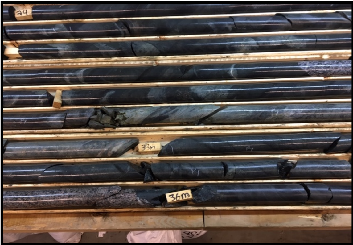
Photograph 4.2.1.1 Main Kakeeway zone veining and alteration.
