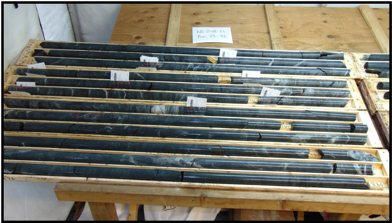
Photograph 4.2.5.5 Silicified and mineralized section 317.10m to 322.24m in drill-hole WL-2018-26.
