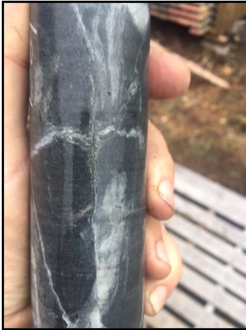
Photograph 4.2.5.3 Pyrite and chalcopyrite as fracture fill drill hole WL-2018-26.
