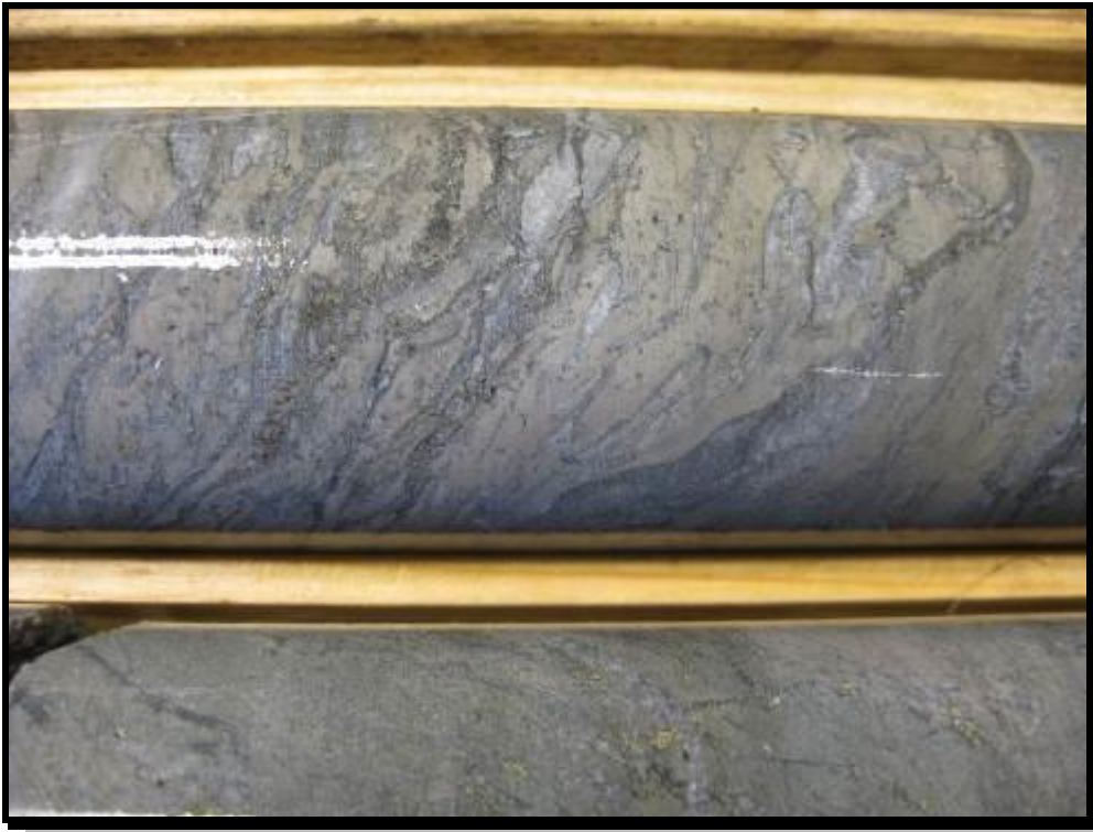
Albite alteration cut by quartz typical of South Zone with pyritization
