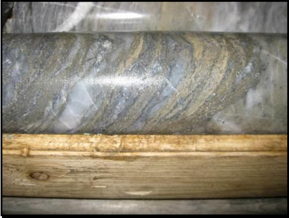
Albite-sericite-carbonate alteration typical of Thomas Ogden Zone with strong pyritization
