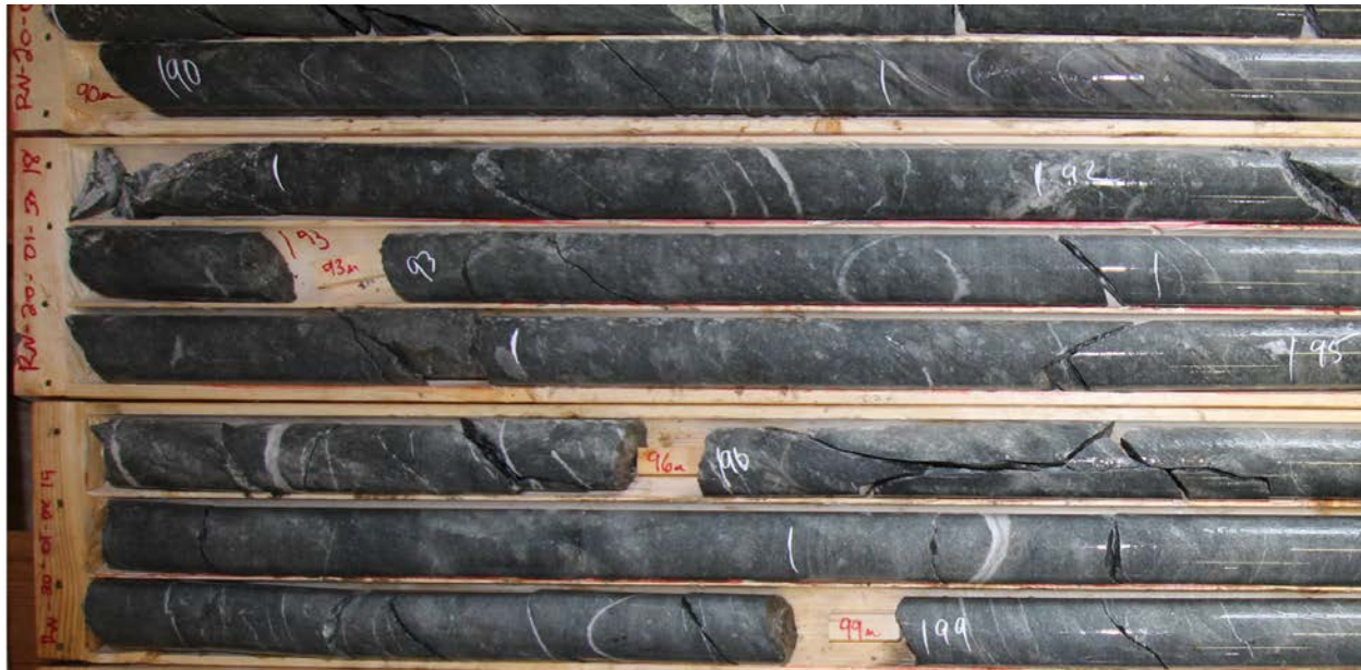
Figure 3: Intermediate Volcanic Tuff (IVOLCtuf) RN-20-01, approximately 93 m downhole. Distinct angular and subrounded clasts up to several cm.
