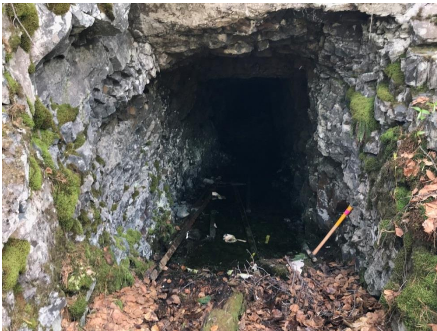
Figure 13: 240 ft adit entrance in greywacke
