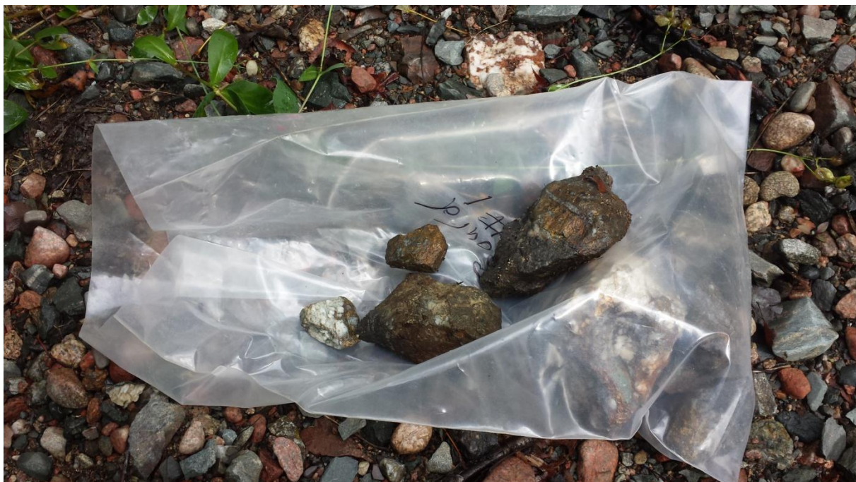
Sample #1, tag B83493 13.3 % Cu., 18ppm Zn., 6.1 ppm Ag.
