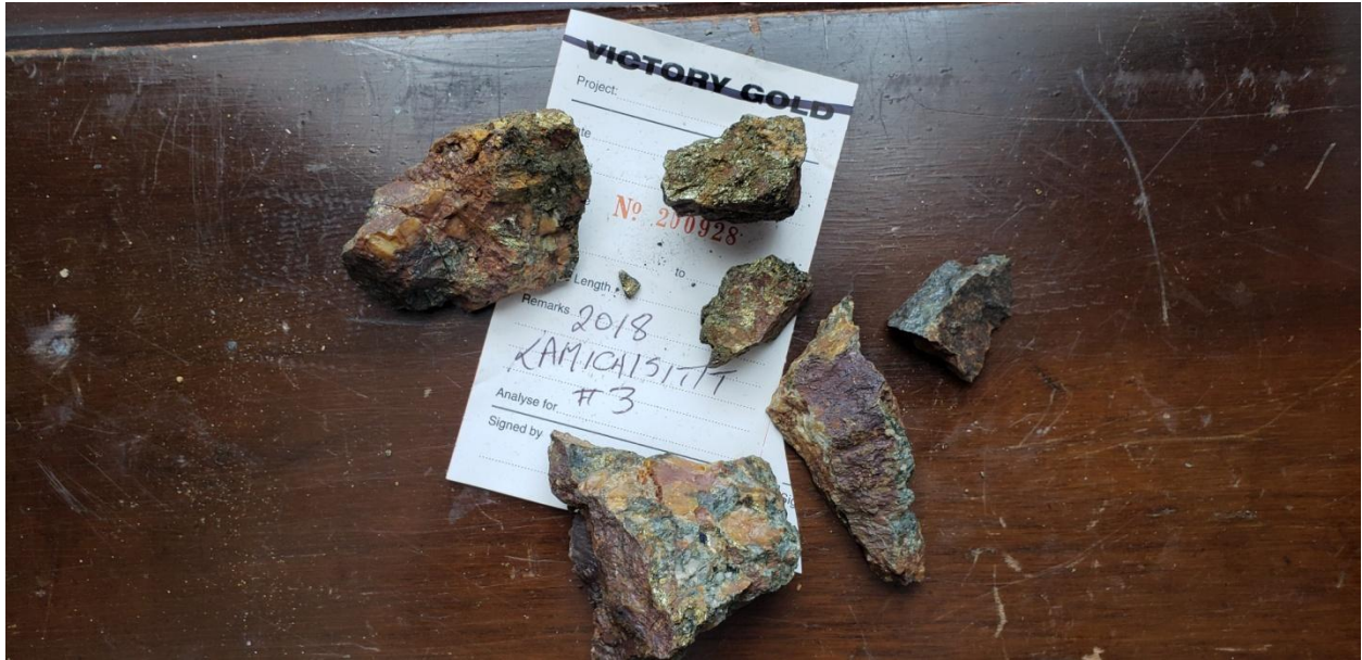
This is sample three, tag # 200928. This sample came from the vein material within a trench located at (17) 343579, 5152865. It tested 3.92% Cu.
