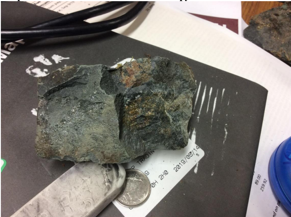
Sample 61 Intermediate volcanic with chalcopyrite blebs
