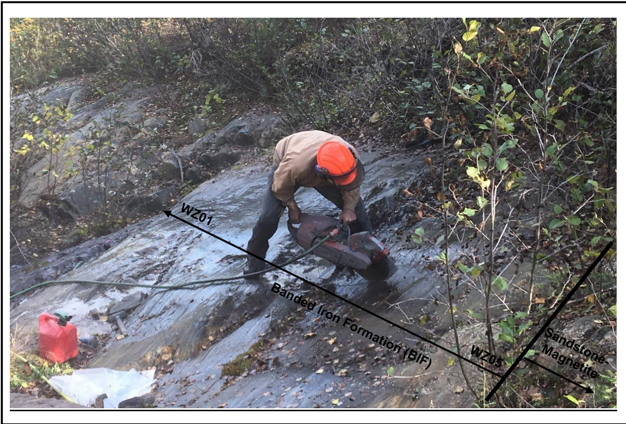
Figure 14: Wilcott Fe Zone photo, AMI Stripping, Oct 2019 – channelling BIF (WZ01 to WZ05)
