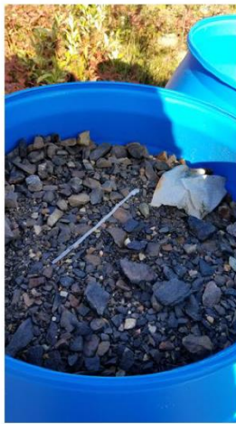
Footwall: ~50-100 m wide 10-30% magnetite BIF with 5-15% clay minerals and 50-60% SiO 2 (Cluster 2)
