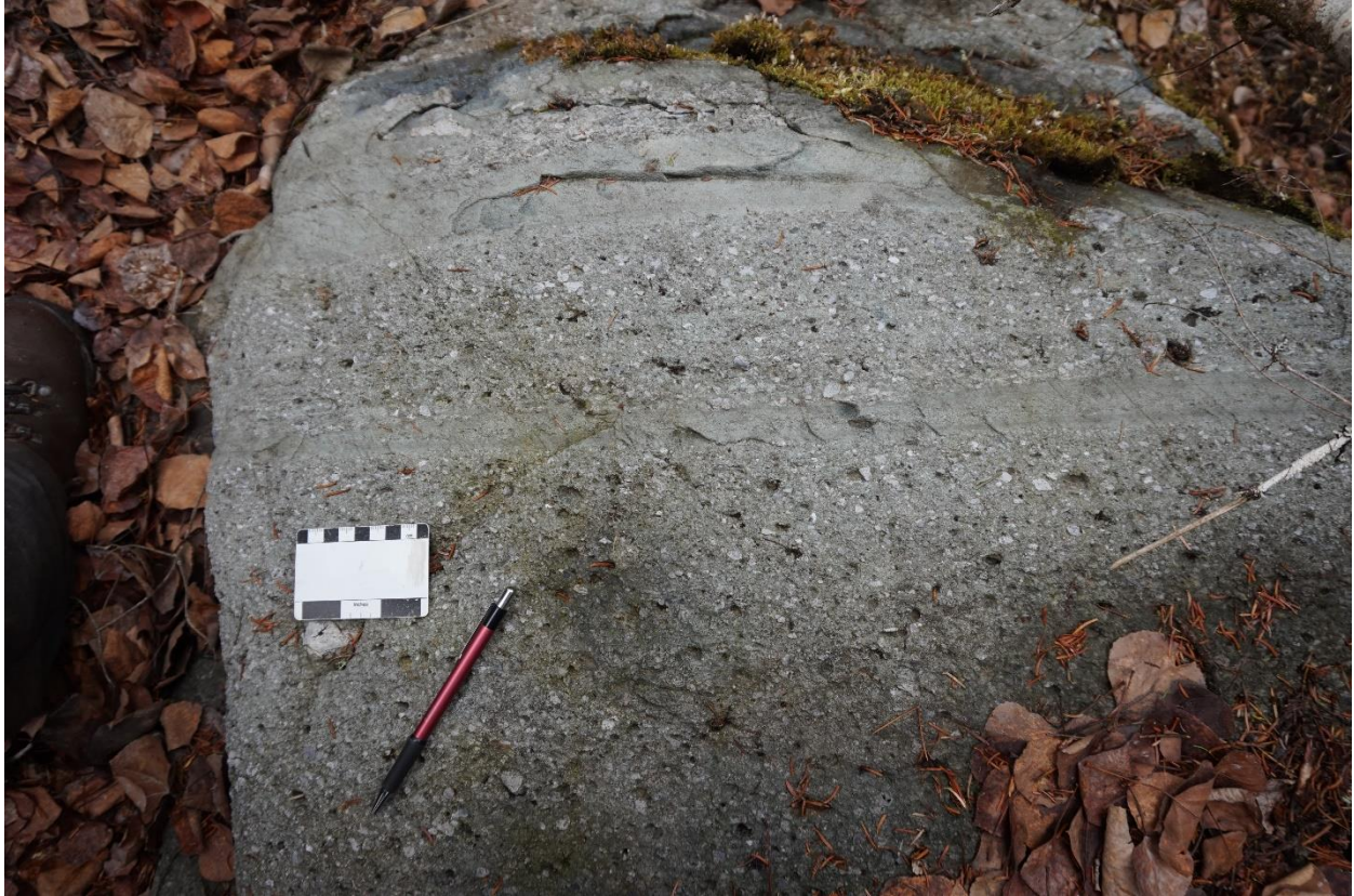
Figure 3: Intermediate volcanoclastic rock with bedding defined by alternating parallel tuffaceous and lapilli tuff layers. Station 19DL017 (UTM NAD83 Zone 15N 509562mE, 5507286mN).
