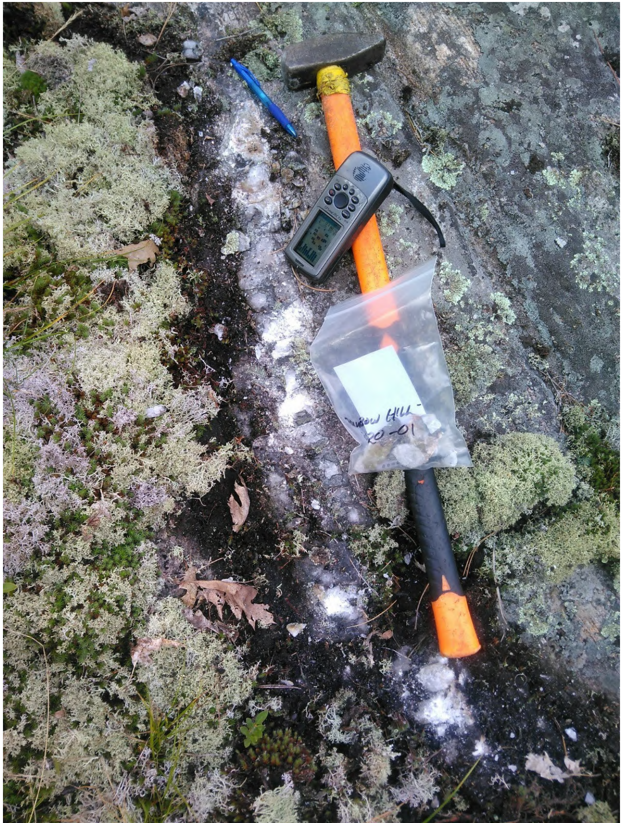
Sample Rainbow Hill-2020-01. Narrow, barren, glassy, quartz vein. Chip sampled over 1 meter.
