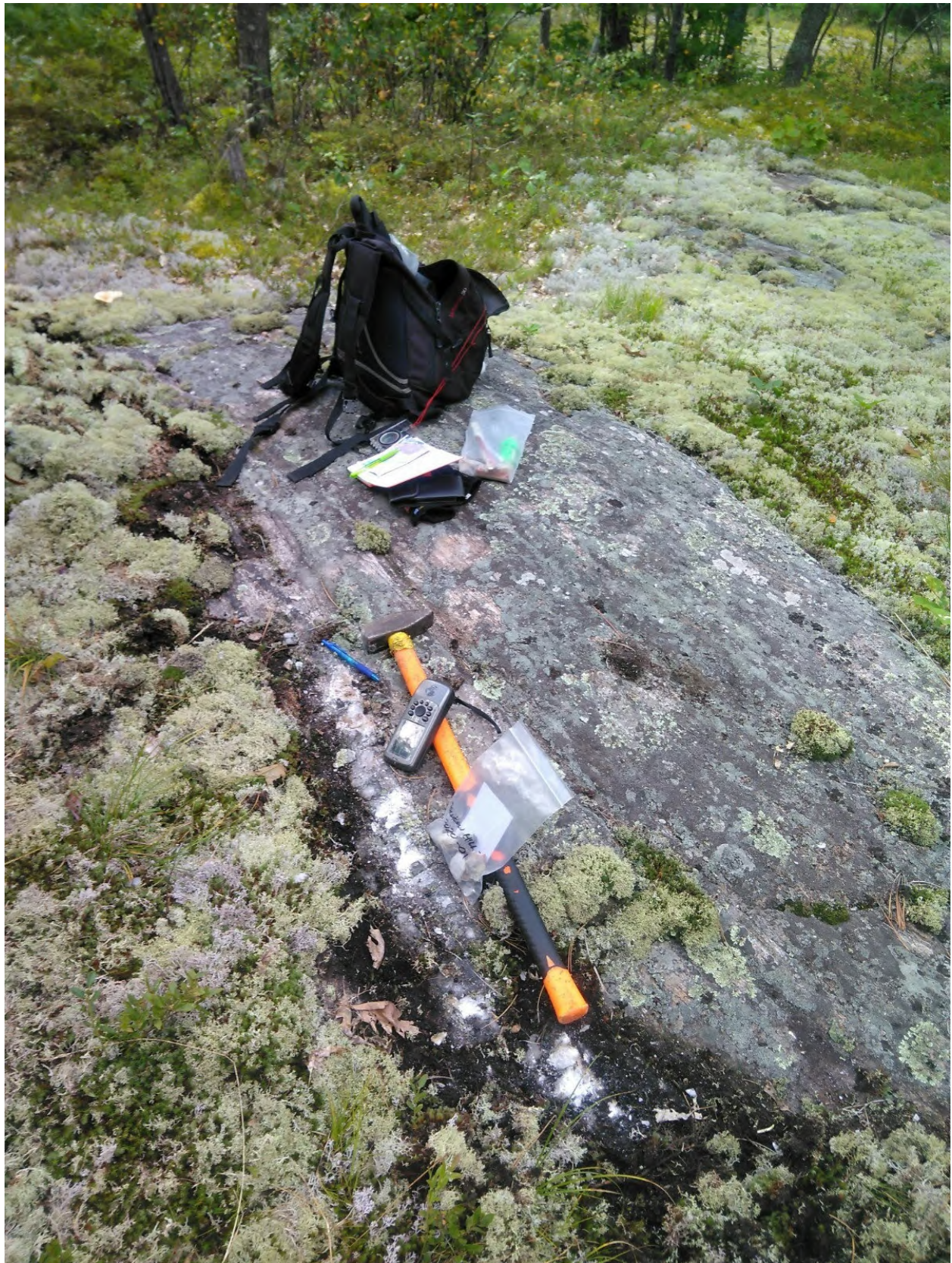
Sample Rainbow Hill-2020-01. Chip sampled over 1 meter. Silica intruded between the bedding planes.
