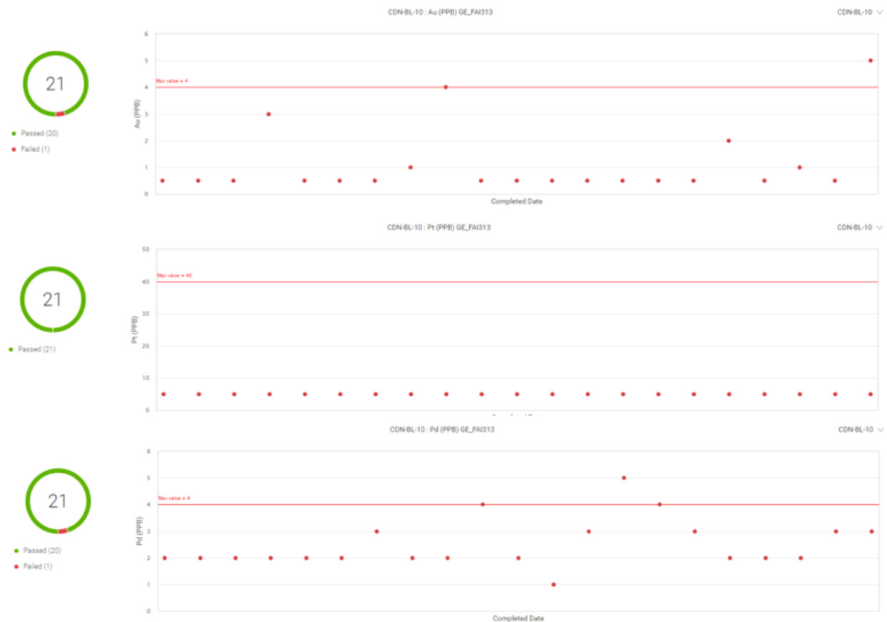
Figure 12: powdered blank analysis for method GE FAI313 (Au, Pt, Pd)
