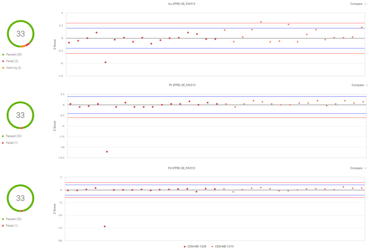
Figure 5: Original assay certificates for all standards including one failed standard. Note that gold values are provisional with the analytical technique used and are therefore deemed as acceptable.
