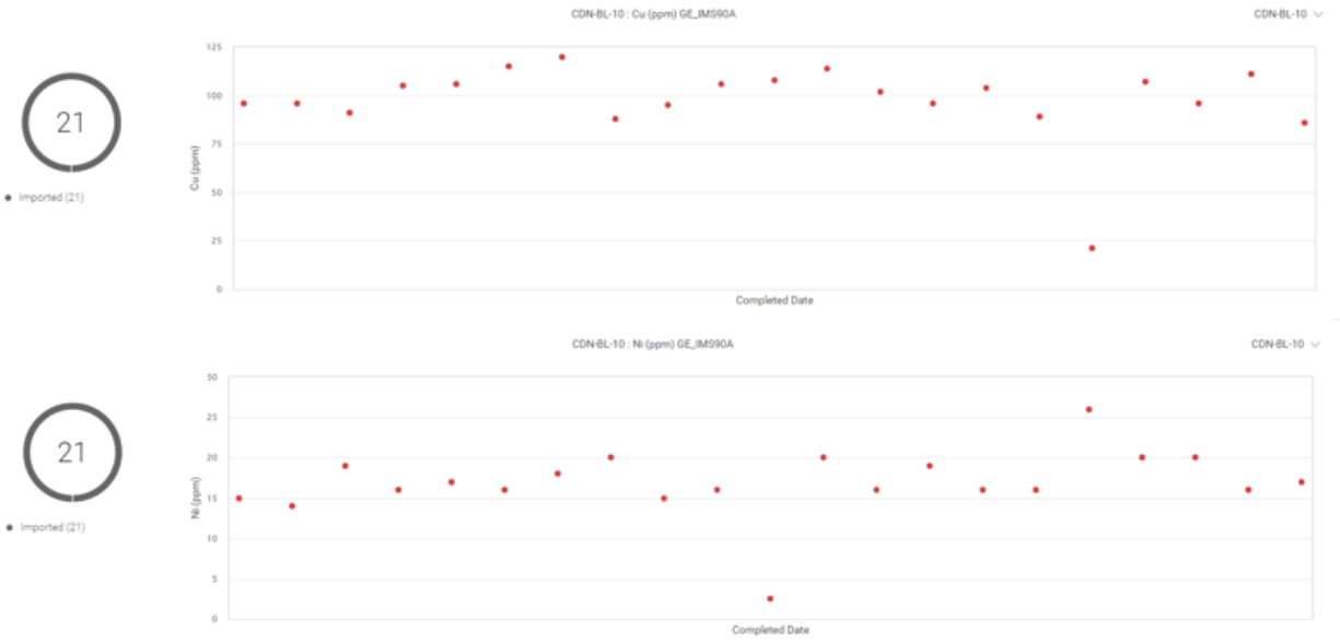
Figure 14: Powdered blank analysis for method GE IMS90A (Cu, Ni)
