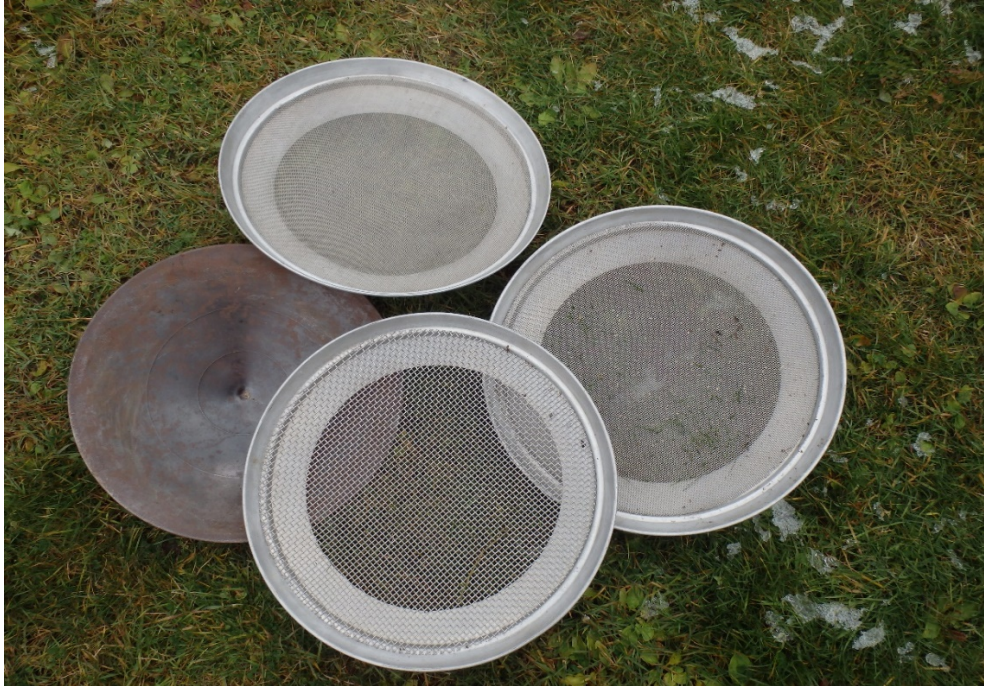
Photo 1 – Screens and pan used to clean and concentrate till/overburden samples
