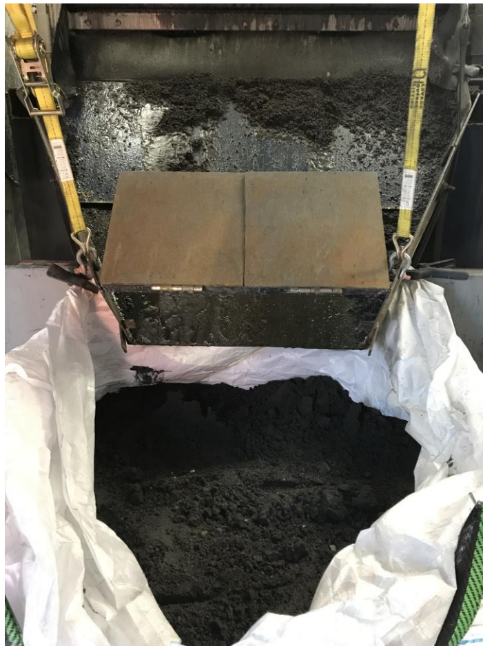
Figure 16: Bulk sample collection in large sample tote from the shaker table
