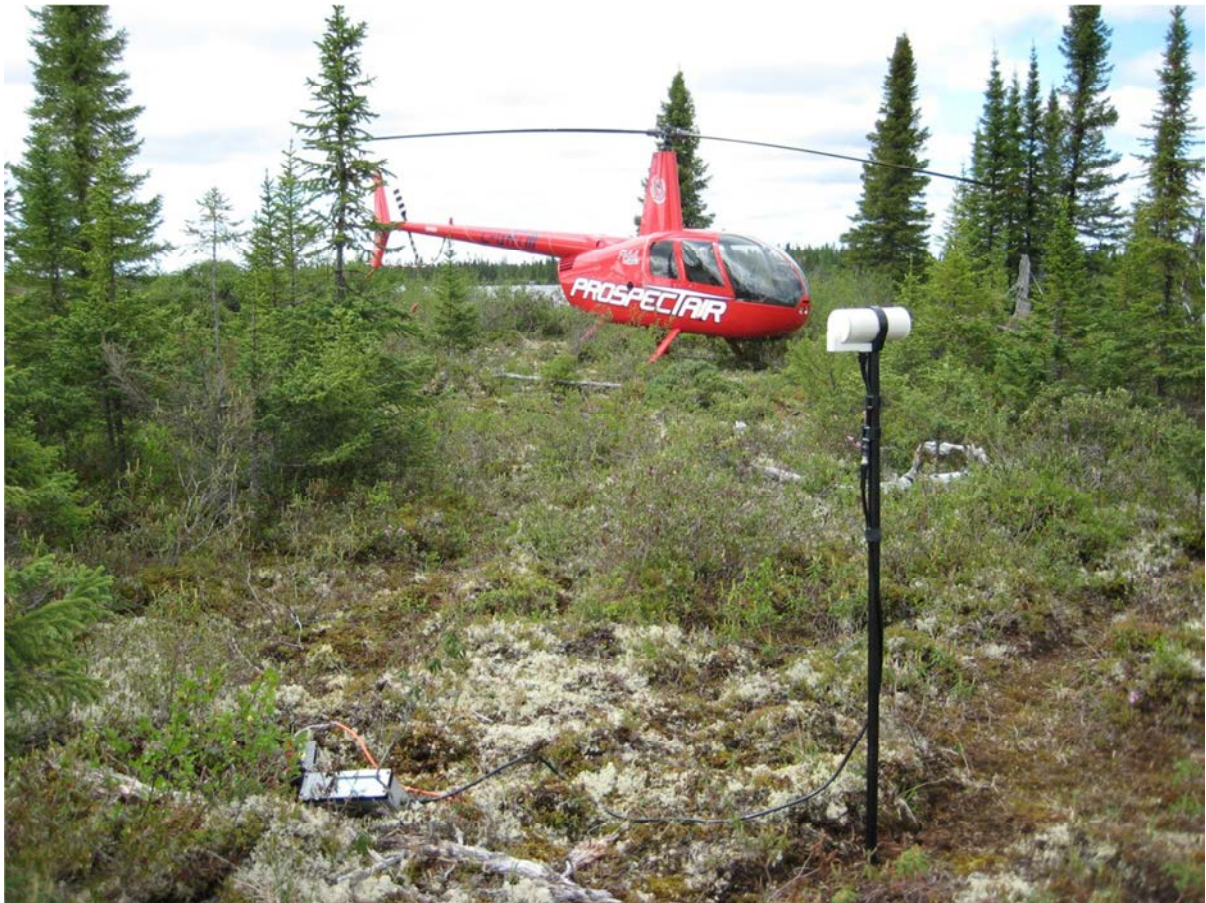
Figure 5: Example of a magnetic base station setup
