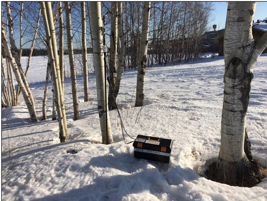
Figure 8 – Base station magnetometer used for diurnal corrections.
