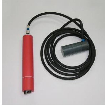
Figure 6 – Scintrex CS-3 magnetometer sensor, cable and electronics.
