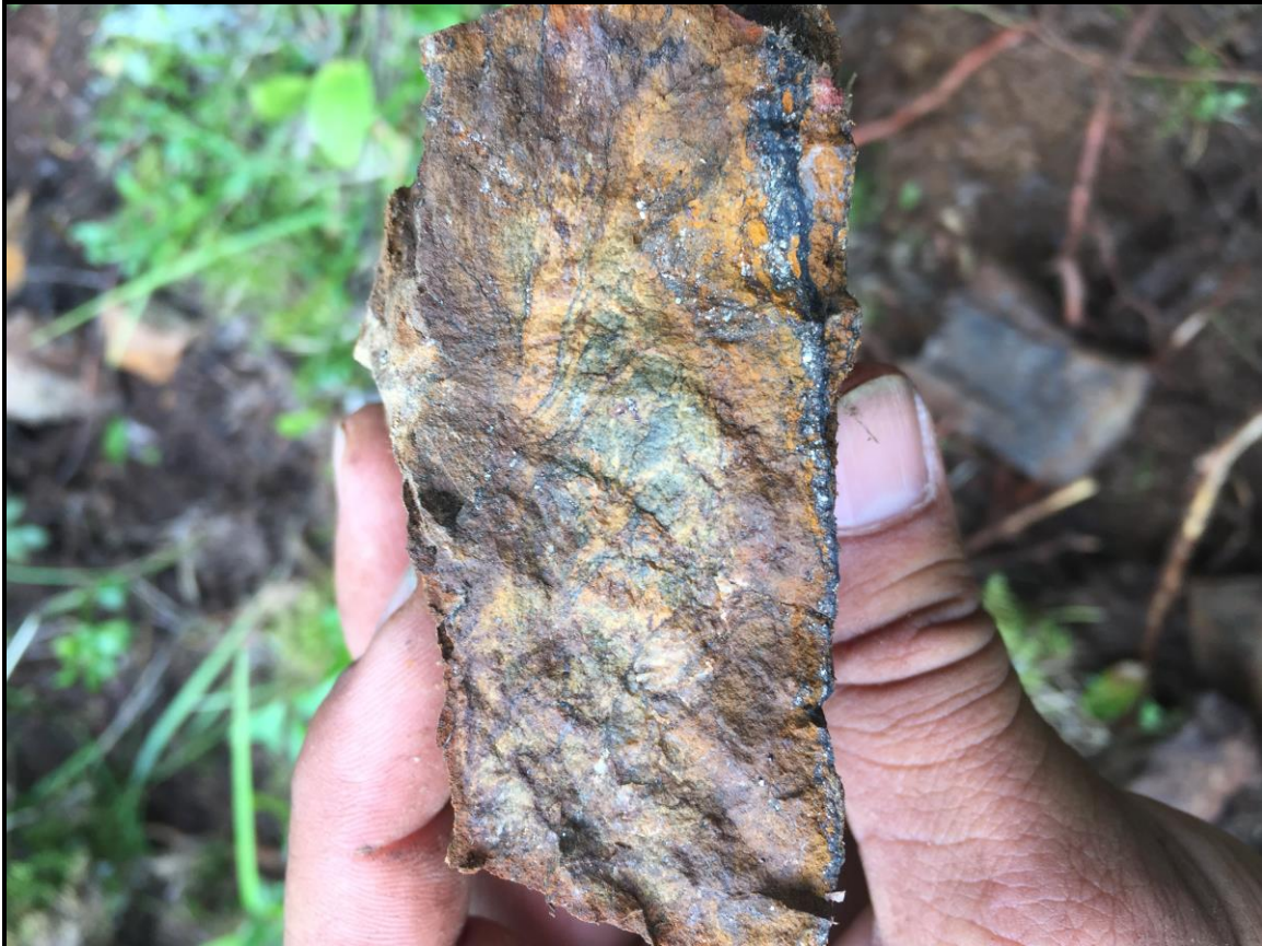
Plate 2: strong carbonate alteration within folded volcanics with stringer pyrite at MM showing (BLMM-20-10)
