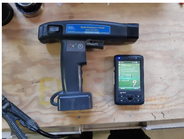
Figure 7: MPP-EM2S+. Magnetic Susceptibility Reader.
