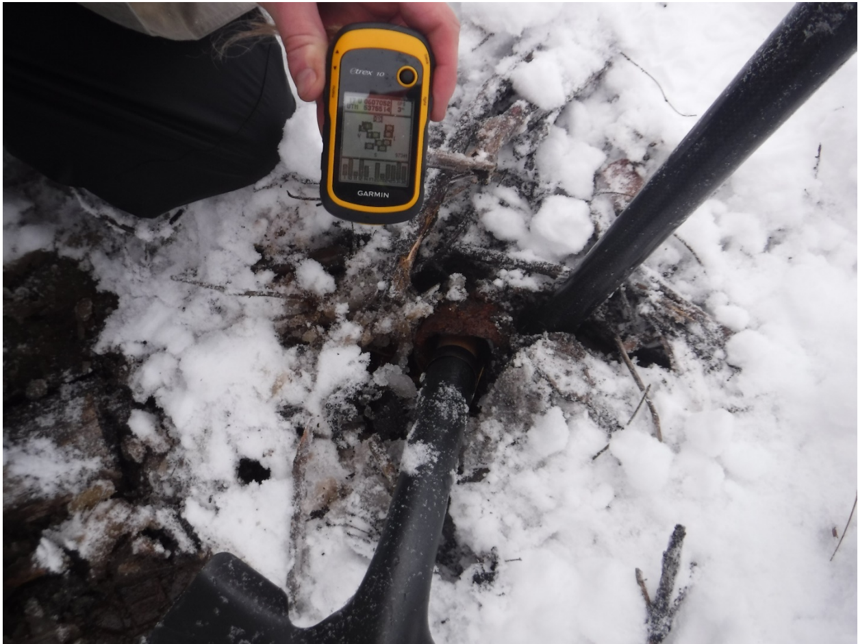
Figure 11-2. Historic drill collar GH95-101 with handheld GPS coordinates
