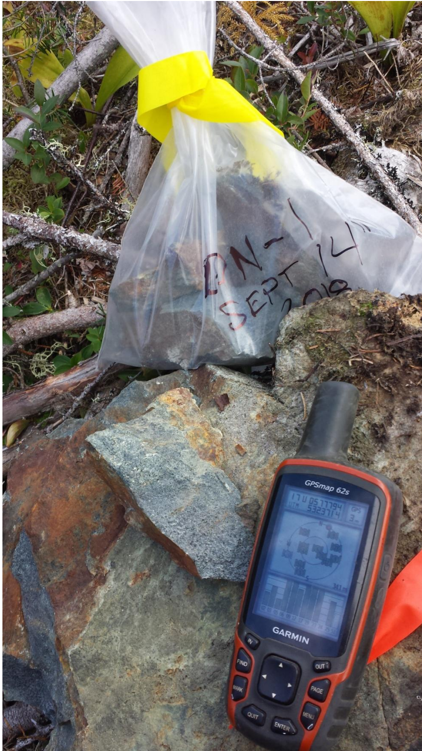
Sample 10 taken from the edge of the new trench prospected on September 14 th , 2018. Rusty with pyrite within the rock.
