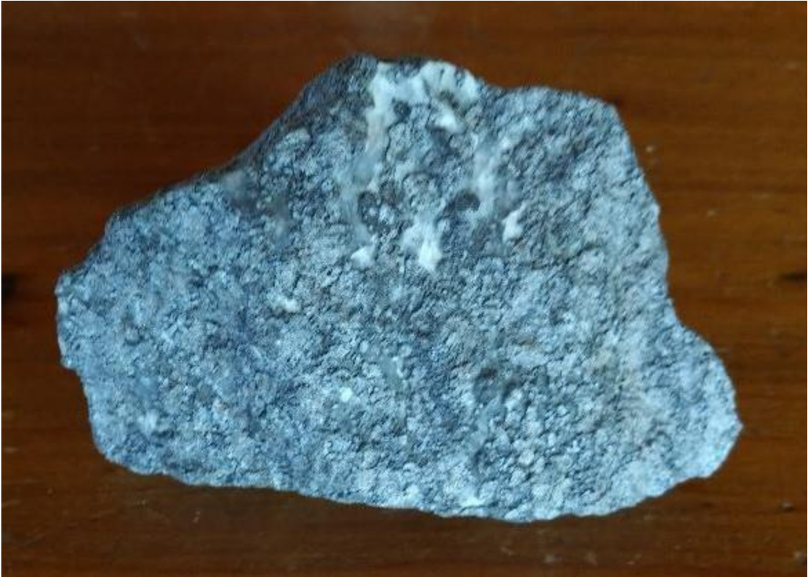
Figure 8.3: Typical specimen of massive cobaltite / smaltite vein material from the Beaver-Temiskaming Mine
