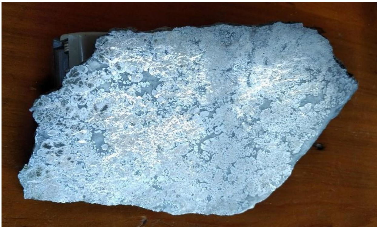
Figure 8.2 illustrates a high-grade native silver in a coliform-textured matrix within a carbonate-Co-Ni arsenide veinlet (10cm wide) sourced from the Beaver-Temiskaming Mine. The grade of this specimen is in the range of 15,000 oz. Ag / tonne.
