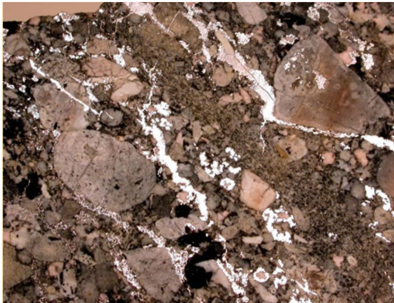
Figure 8.1: Sawn Specimen of Coleman Formation Conglomerate from O'Brien Mine
