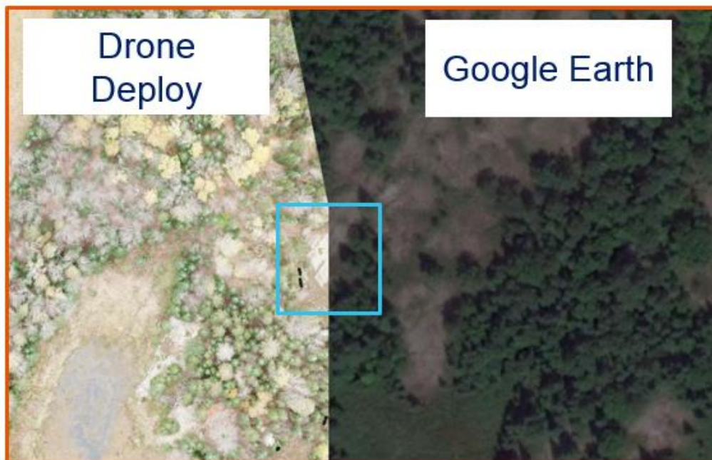
Figure 4: View of inset comparison as shown above, can easily identify exposed uncovered bedrock outcropping, sudden changes in vegetation or topography. Can be very useful in determining future sampling locations.
