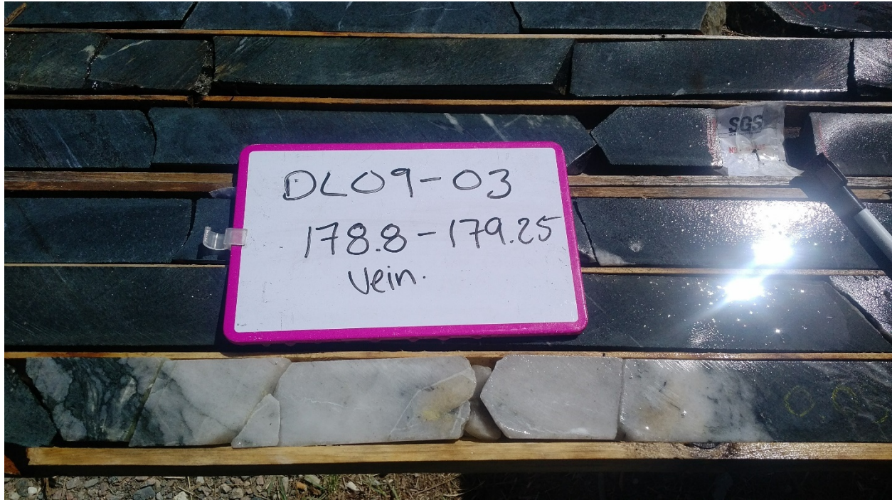
Figure 6: Prospective Quartz Vein from DL-09-03.
