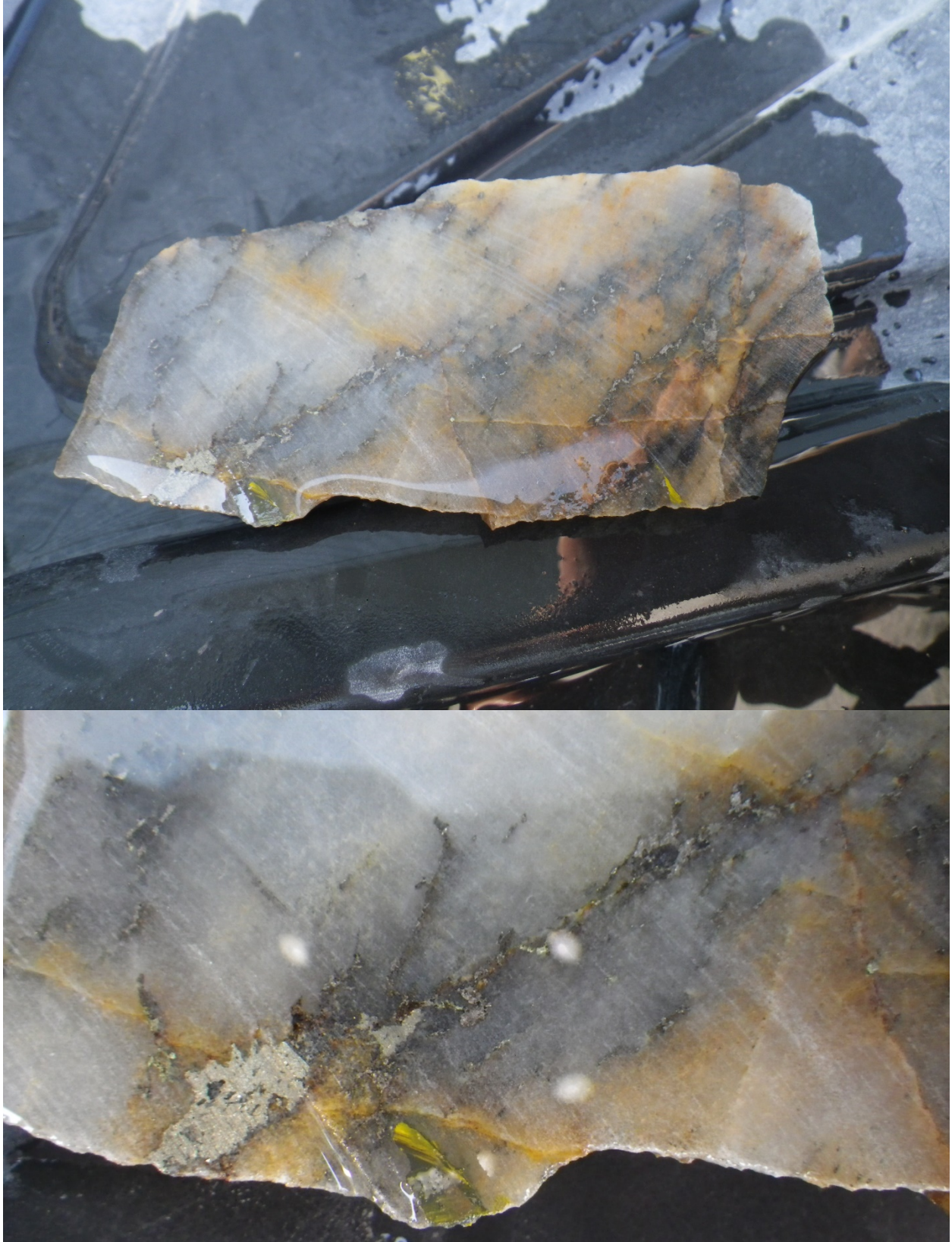
Figure 12: Quartz with close-up of coarse pyrite, and seam of pyrrhotite and chalcopyrite.
