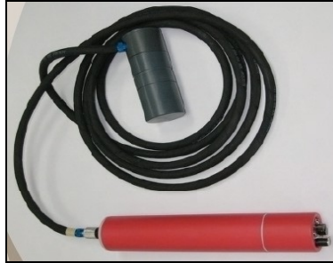
Figure 6: Scintrex CS-3 Cesium Magnetometer.
