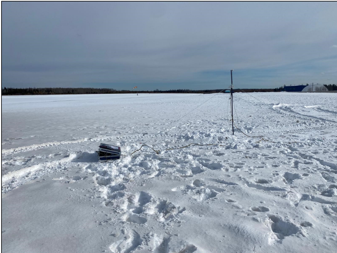
Figure 4: The GEM GSM-19 base-station magnetometer.
