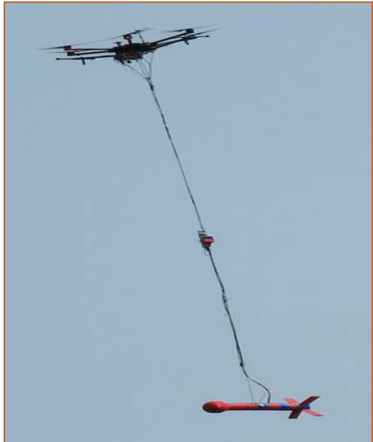
Figure 11. Vision4k UAV-Multirotor with CS-VL magnetometer.
