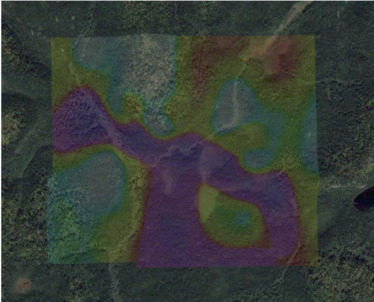
Figure 25: Resistivity grid (250m MSL) overlaying Google Earth. (©2018 Google, Image ©2019 CNES/Airbus, Image ©2019 DigitalGlobe)
