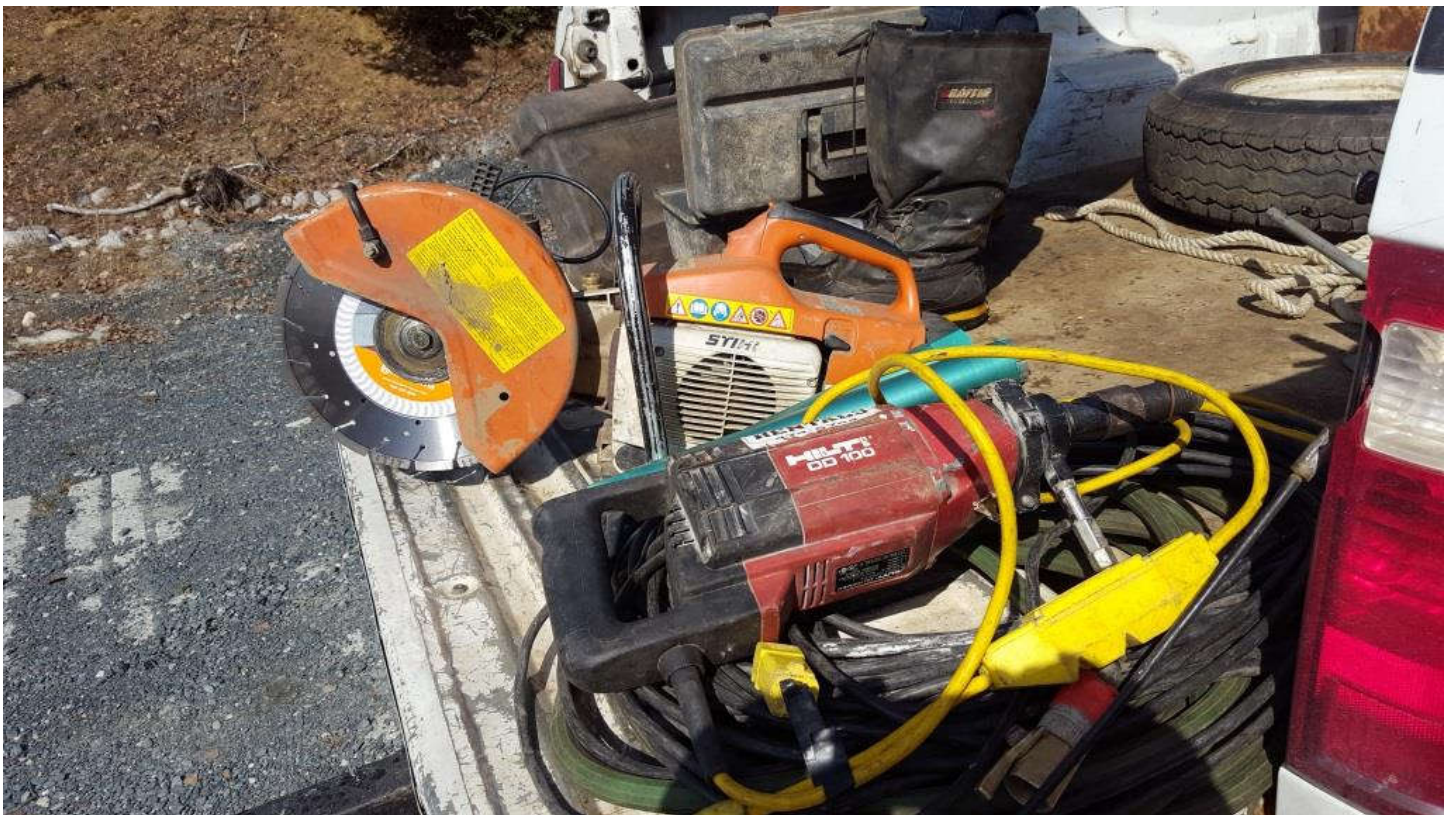
Figure 6: STIHL Rock saw to cut the samples in the field and Hilti Plugger Drill
