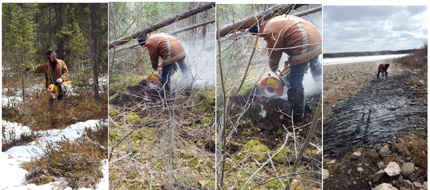
Figure 8: Samples collection with Rock Saw in the field and at 356151 and 356154 locations
