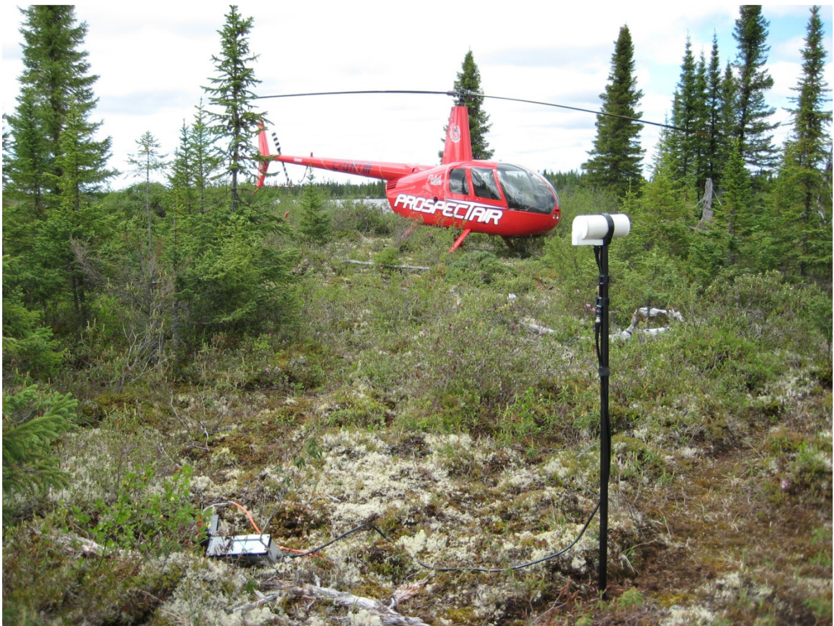
Figure 6: Example of a magnetic base station setup
